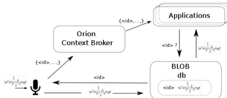
Figure 6: Processing events and saving sound bites to a binary large object (BLOB) storage database.
