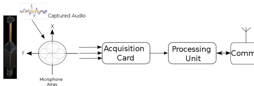
Figure3: FI-Sonic Sound Acquisition Module (Architecture).
