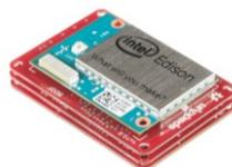
Figure 4: Intel Edison (Top board), as the main Processing Unit.
