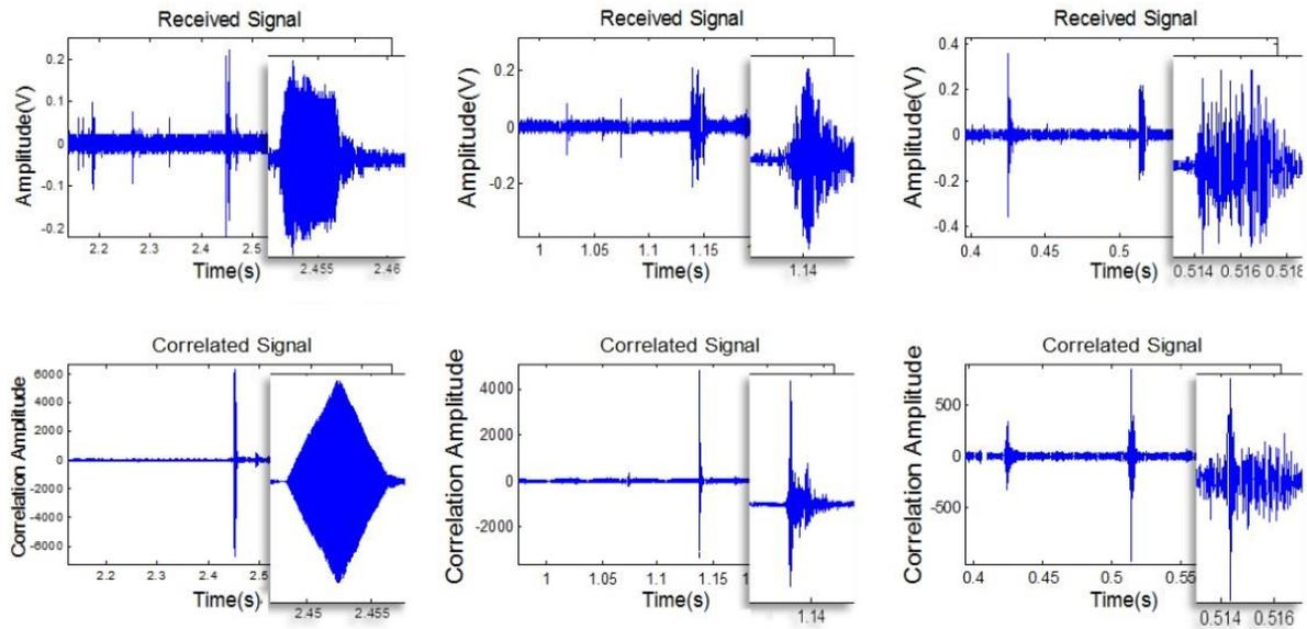
Figure 8. Example of recorded signals at 112.5 m E-R in the harbour of Gandia.
