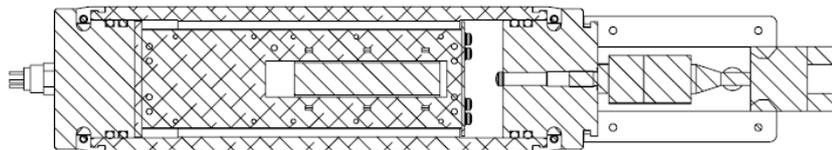
Figure 7. Drawing of the Acoubeacon, internal mechanical structure.
