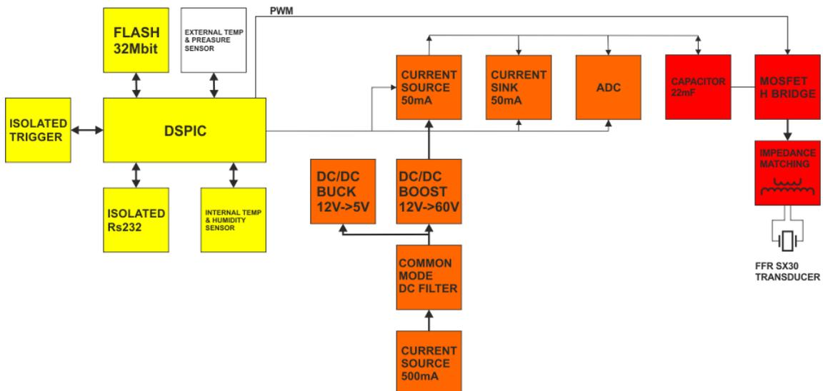
Figure 6. Block diagram of the electronic board
