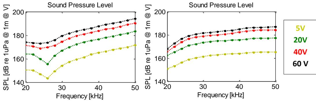
Figure 3. Sound Pressure Level (SPL) of the Acoubeacon at axial direction (left) and radial direction (right) for different capacitor charge.
