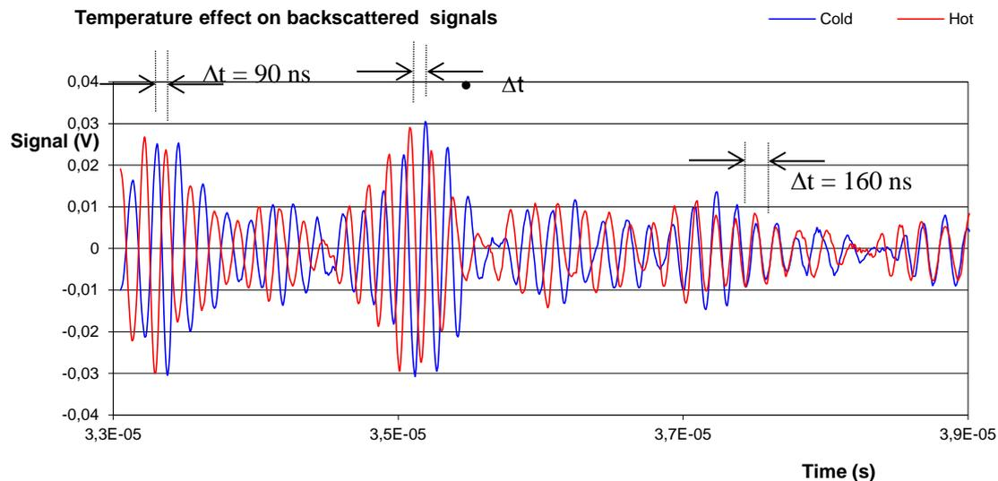
**Figure 1: Backscattered echo-signal before (blue) and after (red) heating. The shift between the signals increases, indicating a temperature rise. The increase per time unit is higher on the right than on the left, indicating a higher temperature rise in the right than on the left (The graph has been taken from the original TNO work)**
