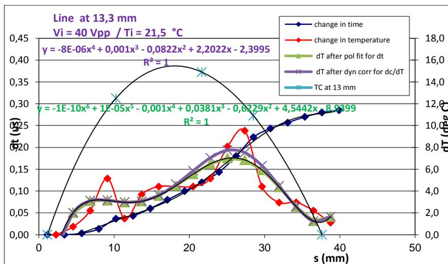
Figure 3: Rise of temperature estimation at 13,3 mm from the phantom top
