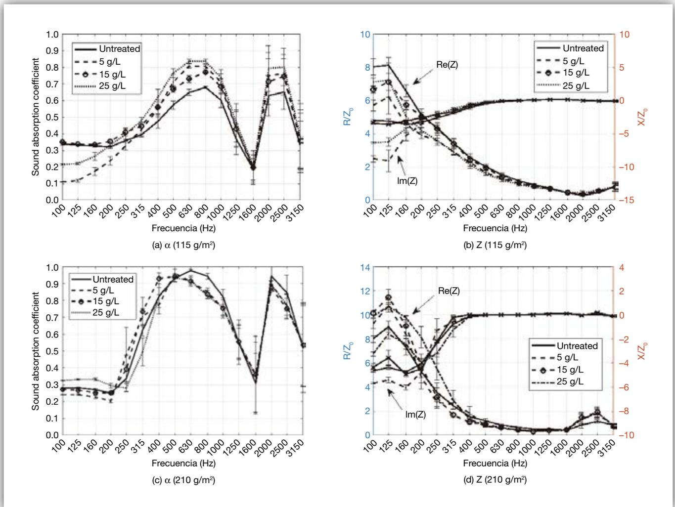
**Figure 5.** Results of the normal incidence sound absorption coefficient and the specific acoustic impedance of the CO fabrics with different saturations of doping are presented. Also, measurements considering the thickness of an air cavity of 10 cm behind the cotton sample studied. The dispersion percentage is measured in order to study the variability of the data and it is expressed as error bars.
