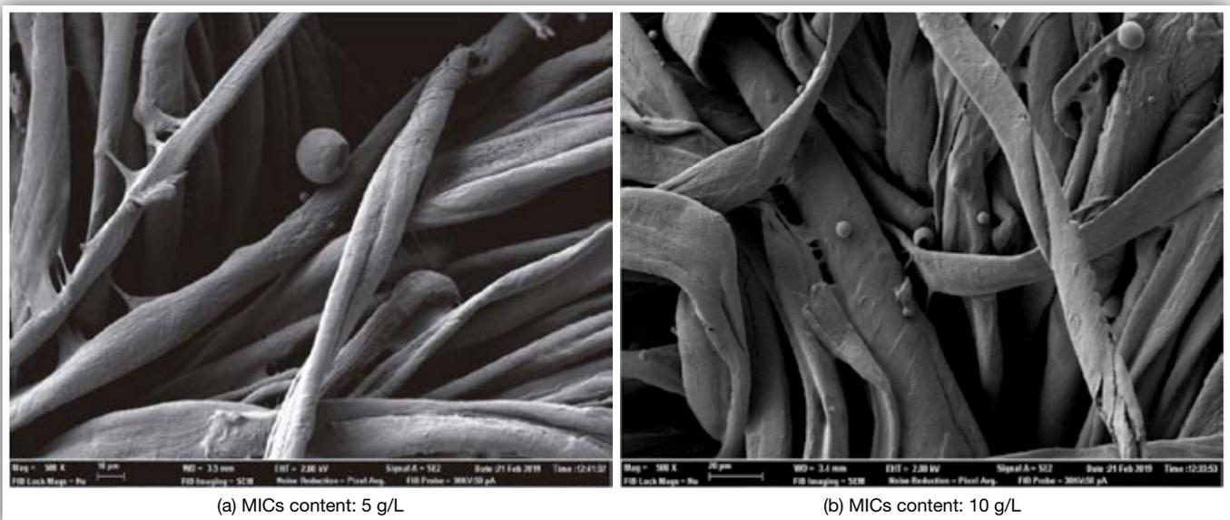
**Figure 2.** FESEM micrographs of cotton fabrics examined with suitable accelerating voltage of 2 kV and 500X magnifications. (a) Sample surface of CO fabric doped with MICs content of 5 g/L; (b) Sample surface of CO fabric doped with MICs content of 10 g/L.
