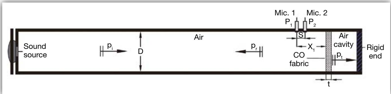
**Figure 3.** Schematic diagram of the impedance tube with an air-cavity of 10 cm used to measure the normal incidence sound absorption coefficient in accordance with the standard ISO 10534-2:1998.  $D$  is the tube inner diameter,  $p_i$  is the sound pressure of the incident wave,  $p_r$  is the sound pressure of the reflected wave,  $p_t$  is the sound pressure of the transmitted wave, and  $t$  is the sample thickness.
