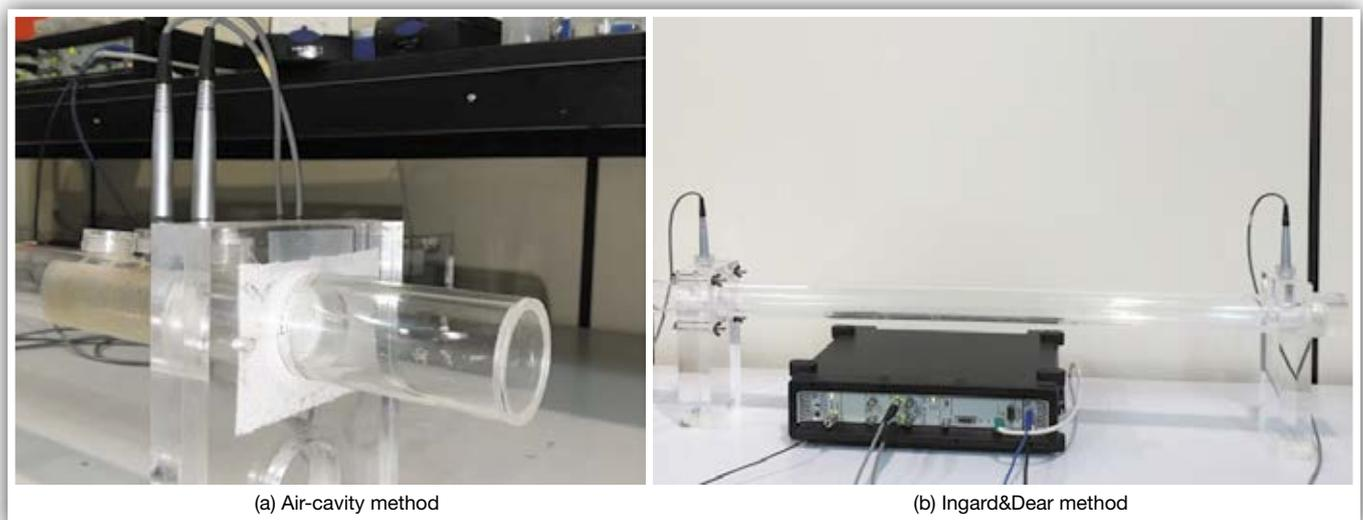
**Figure 4.** Experimental setup using the impedance tube. (a) Measurement of normal incidence sound absorption coefficient with an air-cavity; (b) Measurement of the airflow resistance according to Ingard&Dear method.
