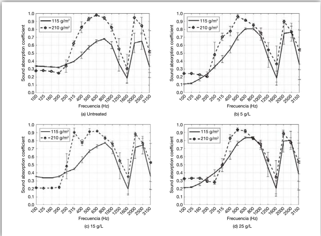
**Figure 6.** Normal incidence sound absorption coefficient of the cotton textile fabric with different yarn densities. Also, measurements considering the thickness of an air cavity of 10 cm behind the cotton sample studied. Error bars expressed the deviation percentage of the measures.
