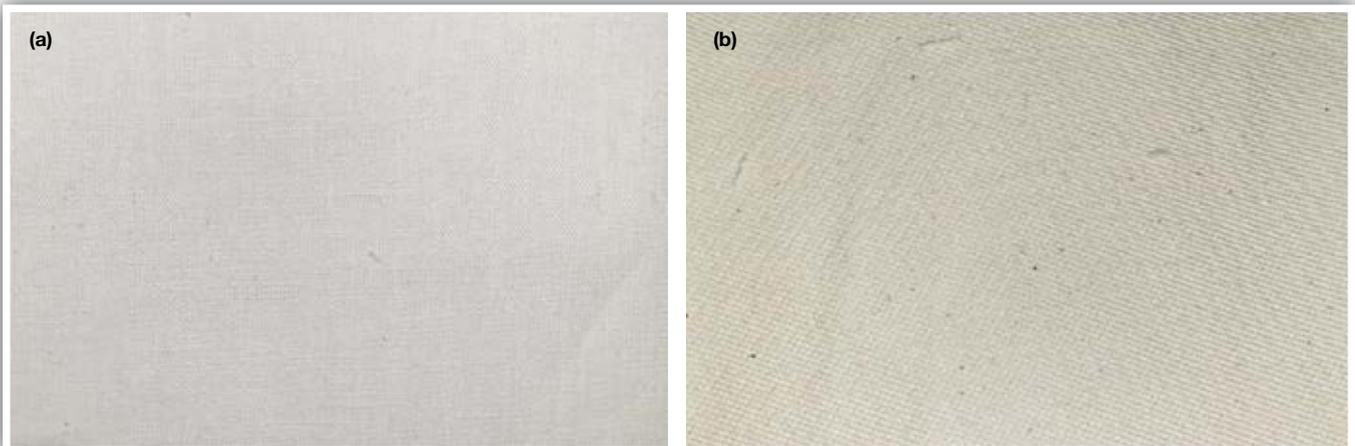
**Figure 1.** Cotton textile fabrics used in this study. Left: CO fabric with a yarn density of 115 g/m<sup>2</sup>; Right: CO fabric with a yarn density of 210 g/m<sup>2</sup>.
