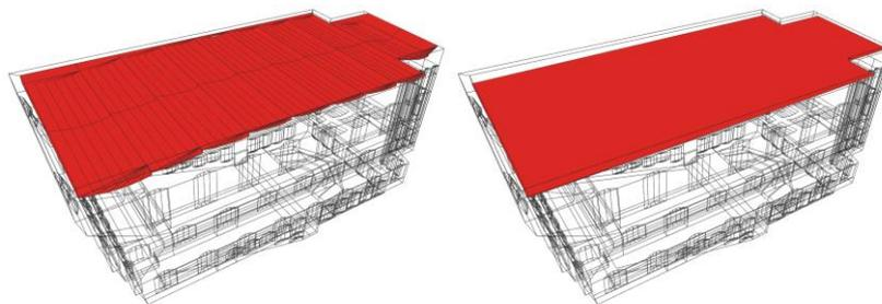
Figure 2 – Example showing the simplification of the ceiling area for a concert hall
