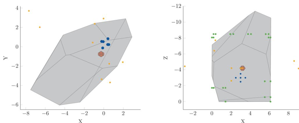
Figure 3 – Results of inverse geometry estimation method of a seminar room. Left figure shows the geometry estimation based on measured RIR, on the right the estimated geometry is based on a simulated RIR. Blue dots indicate the receiver positions, yellow dots detected image sources and green dots show vertices of the original simulated model.
