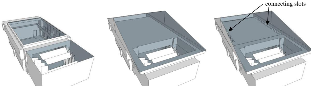
Figure 5 – Three models of a chamber music hall in Berlin. Left model only contains the main room and the stage, in the middle model, the attic was added (connected via the stage area), in the third model on the right hand side, connecting slots (for lighting) were added to the model. Ceiling parts are hidden in all models.
