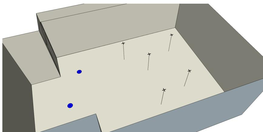
Figure 4 – Room model of seminar room determined with the VariSphere measurement system. Blue circles indicate the sound source positions; Black crosses show the microphone positions
