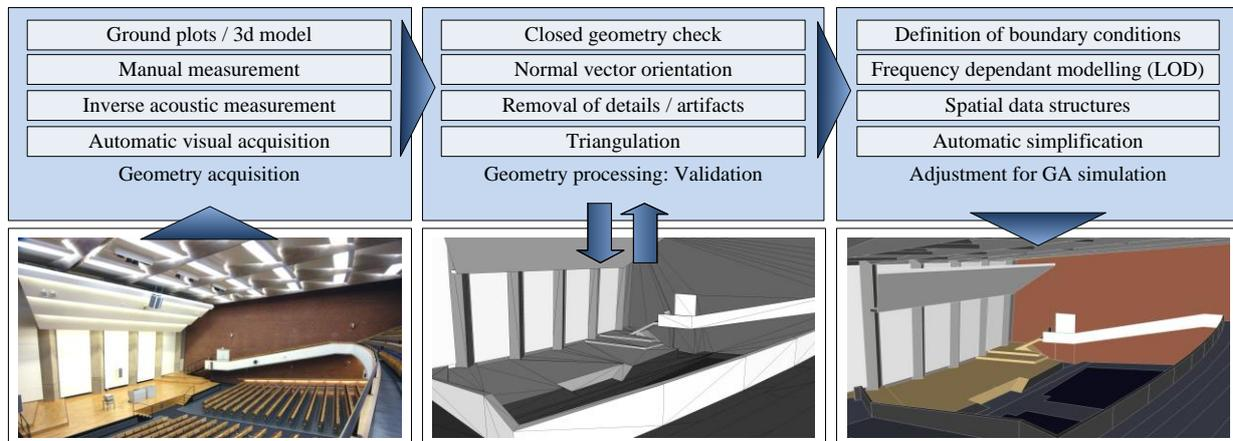
Figure 1 - Geometry acquisition and processing options for a GA-based room acoustical simulation
