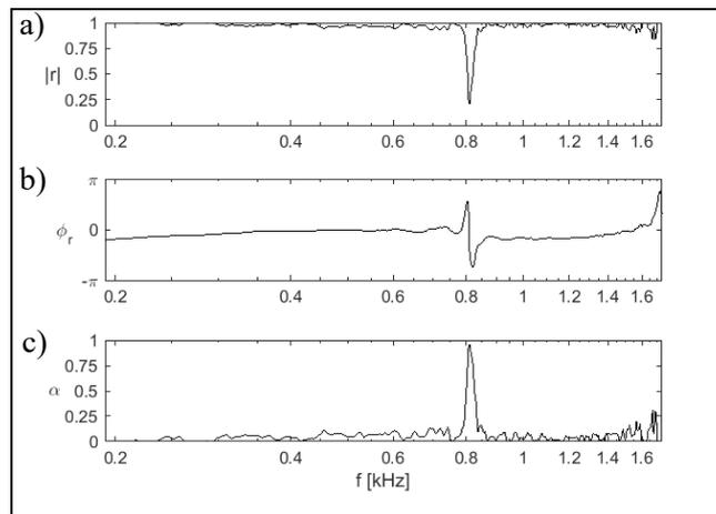
Figure 2 – Experimental measurements considering the air cavity of  $d=0\text{cm}$  ( $|r|$ ). a) Sound reflection coefficient ( $\phi_r$ ), b) Phase of the sound reflection coefficient, c) Sound absorption coefficient ( $\alpha$ ).
