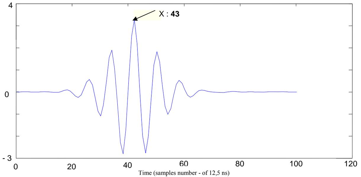
Figure 3. Cross-correlation of first echoes in the two A-Scans (coming from the interface fluid-wall)
