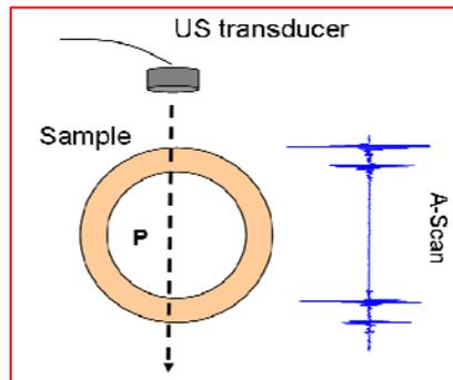
Figure 1. Scheme of the walls displacements measurement in a cylindrical tube.
