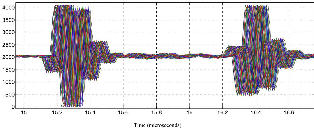
Figure 2. Waveforms of 150 echoes coming from the first wall of a latex tube, for distinct pressures.
