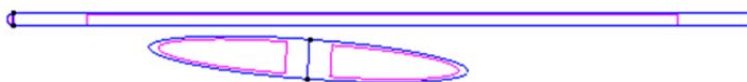
Figure 2. Scheme of fish structure. Swimbladder is approximated as a prolate spheroid and fish bone as a cylinder with smooth edges.
