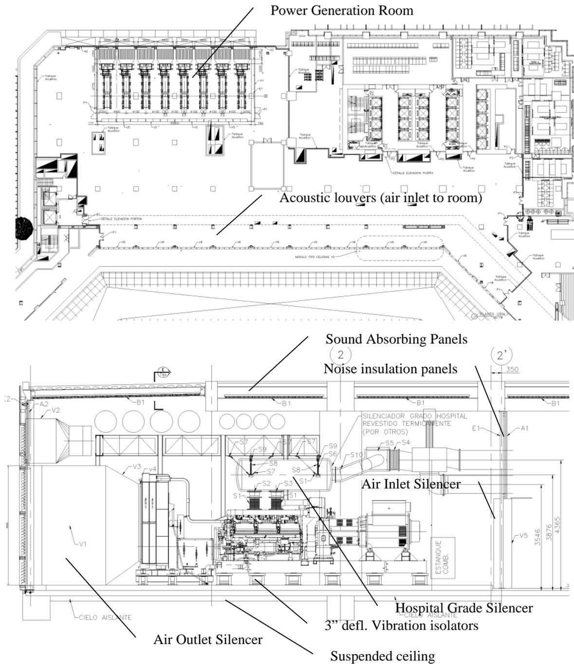
Figure 8 – Center Mechanical room, a) Plan view, b) Section view.
