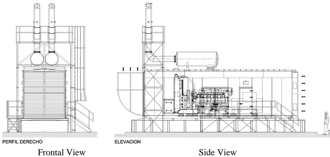
Figure 6 – HP Data Center Enclosure.a) Plans.
