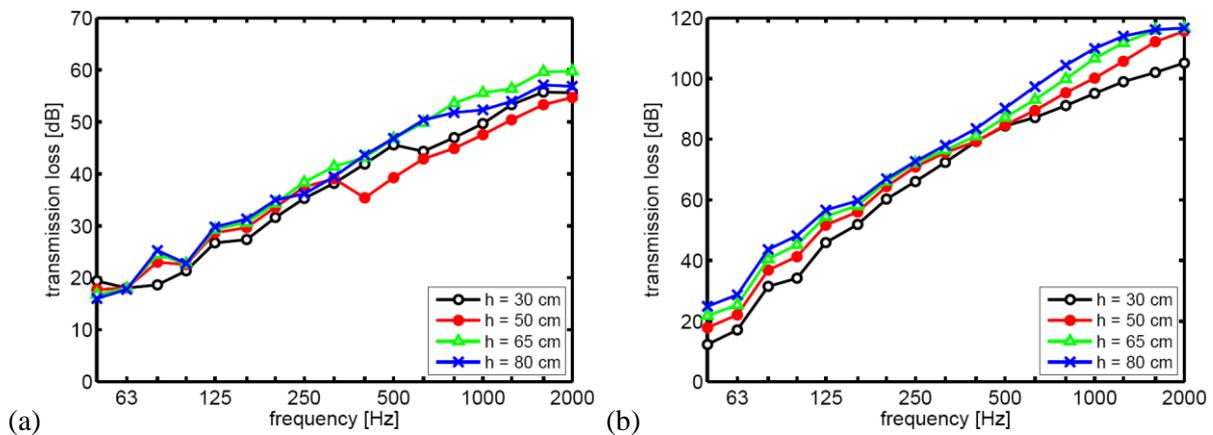
Figure 6 – Influence of the plenum height on the TL of the airborne flanking path across a suspended ceiling with (a) empty plenum and (b) mineral wool in the plenum (filling ratio 30 %).
