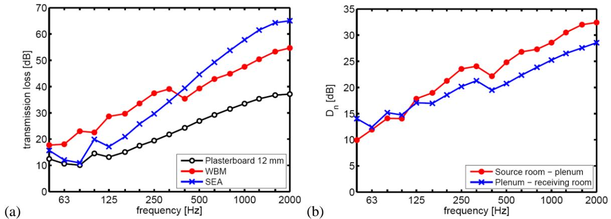
Figure 2 – (a) TL of the airborne flanking path across a suspended ceiling without cavity absorption and (b) normalized sound pressure level differences between rooms and plenum.
