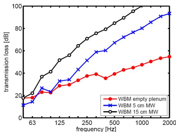
Figure 4 – TL of the airborne flanking path across a suspended ceiling with empty plenum, 5 cm or 15 cm cavity absorption modeled as equivalent fluid (Delany-Bazley model,  $\sigma = 5000$  Ns/m<sup>4</sup>).
