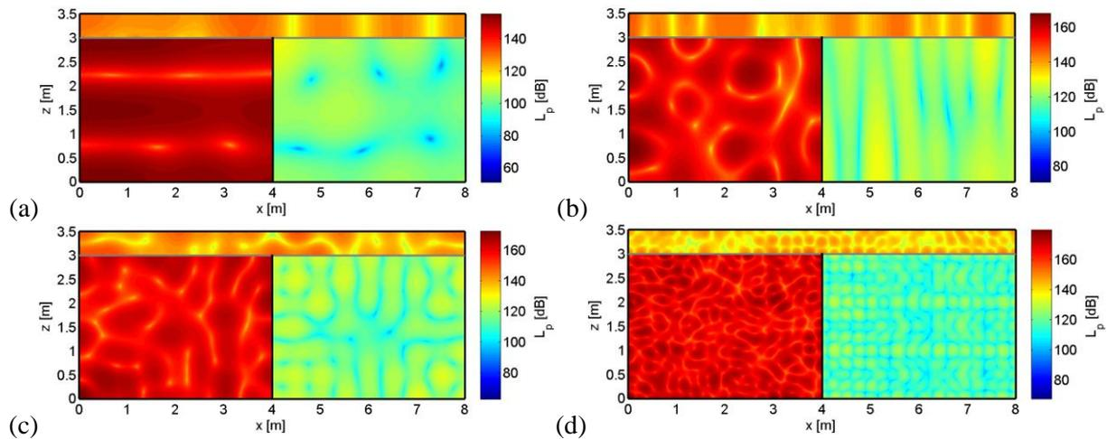
Figure 3 – Sound pressure level distribution in the plane  $y = 1$  m at a frequency of (a) 125 Hz, (b) 300 Hz, (c) 400 Hz and (d) 1000 Hz for the suspended ceiling without cavity absorption.
