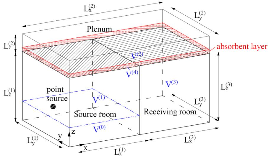
Figure 1 – Geometry of the wave based model: a suspended ceiling with or without cavity absorption above two rooms with rigid side and back walls.
