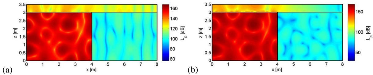
Figure 5 – Sound pressure level distribution in the plane  $y = 1$  m at a frequency of 300 Hz for the suspended ceiling with (a) 5 cm cavity absorption and (b) 15 cm cavity absorption.
