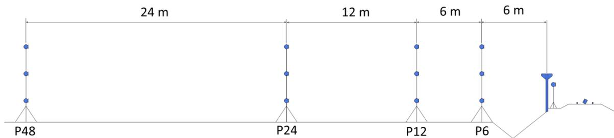
Figure 5 – Sketch of the positions of the measurement points on the protected side
