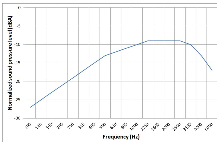
Figure 7 – Normalized railway noise spectrum [7]
