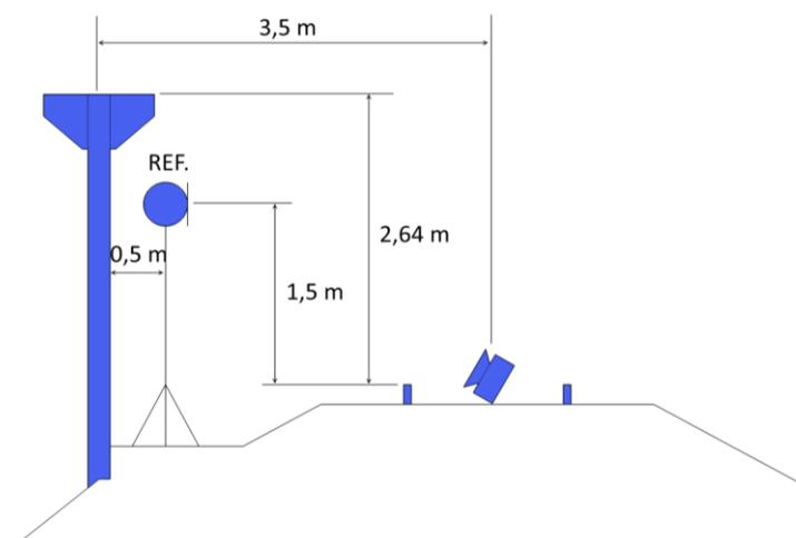
Figure 3 – Measurement setup at the source side of the barrier
