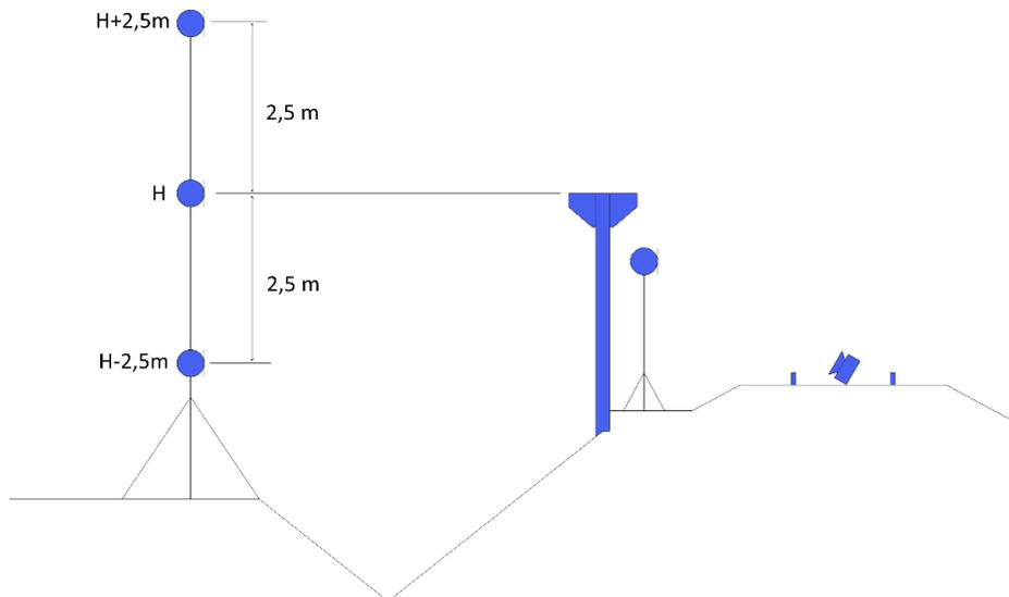
Figure 4 – Sketch of the measurement setup at the protected side of the barrier
