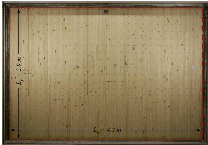
Figure 2 – Cross laminated timber plate installed in a rigid frame in Empa's wall sound insulation test facility
