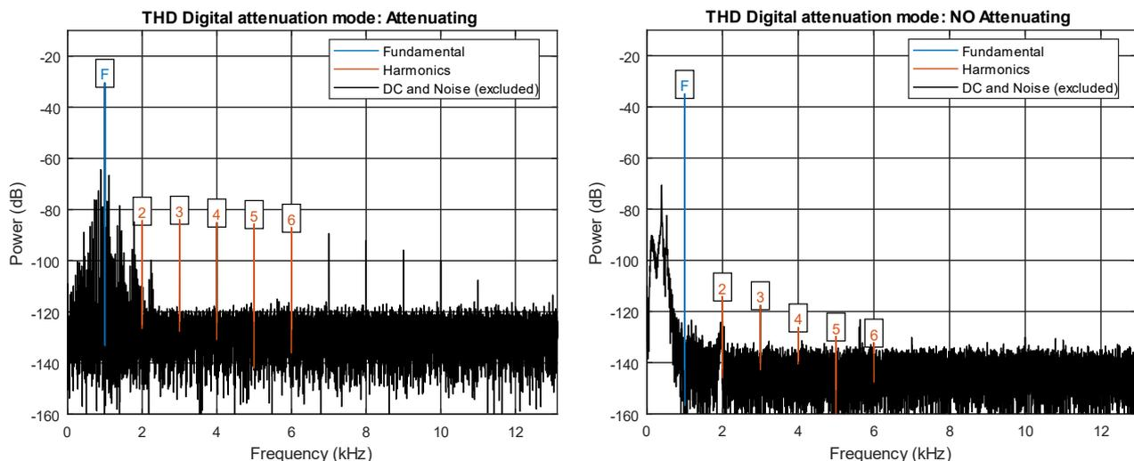
FIGURE 6. Signal to Noise Ratio (SNR) and Total Harmonic Distortions (THD) on a digital limiter implementation with filters acting and not acting on the audio signal.
