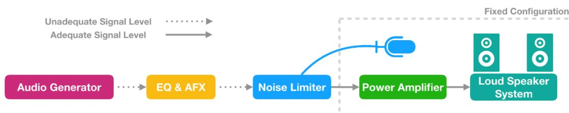
**FIGURE 1.** Acoustical noise limited audio chain.
