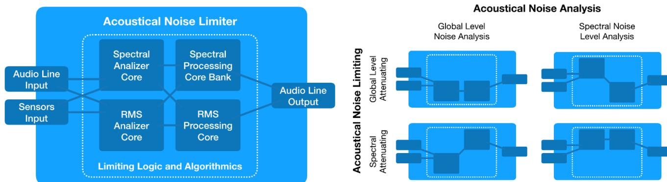
FIGURE 3. Acoustical noise limiter key blocks and basic configurations.
