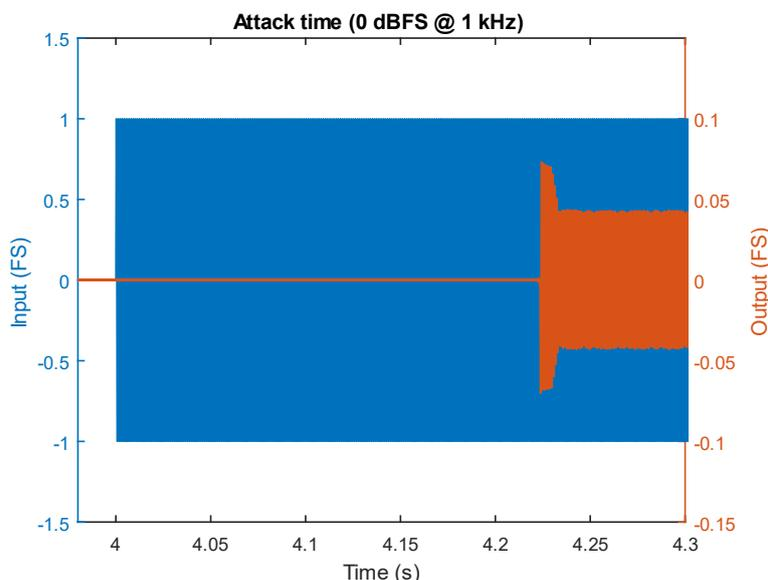
FIGURE 4. Attack time and input to output delay measured on a digital acoustical noise limiter.
