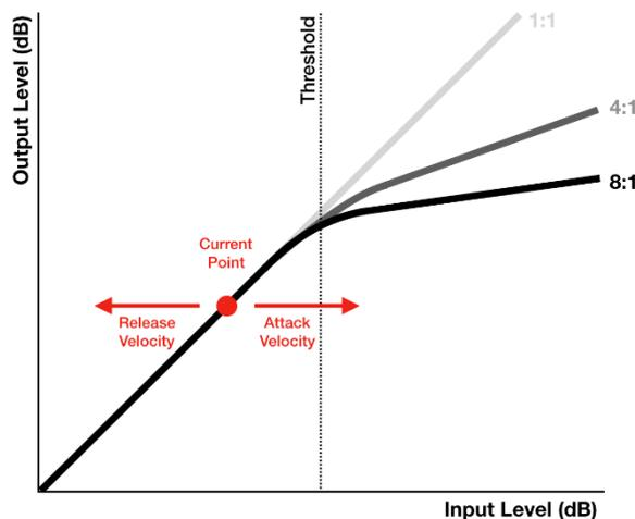
FIGURE 2a. Compressor input-output diagram.
