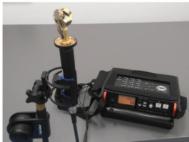
Fig. 5. Ambisonic microphone Sennheiser AMBEO VR MIC and Tascam DR-680 MkII multi-channel digital recorder.
