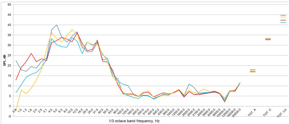
Fig. 3. Results of background noise measurements in the acoustic chamber.
