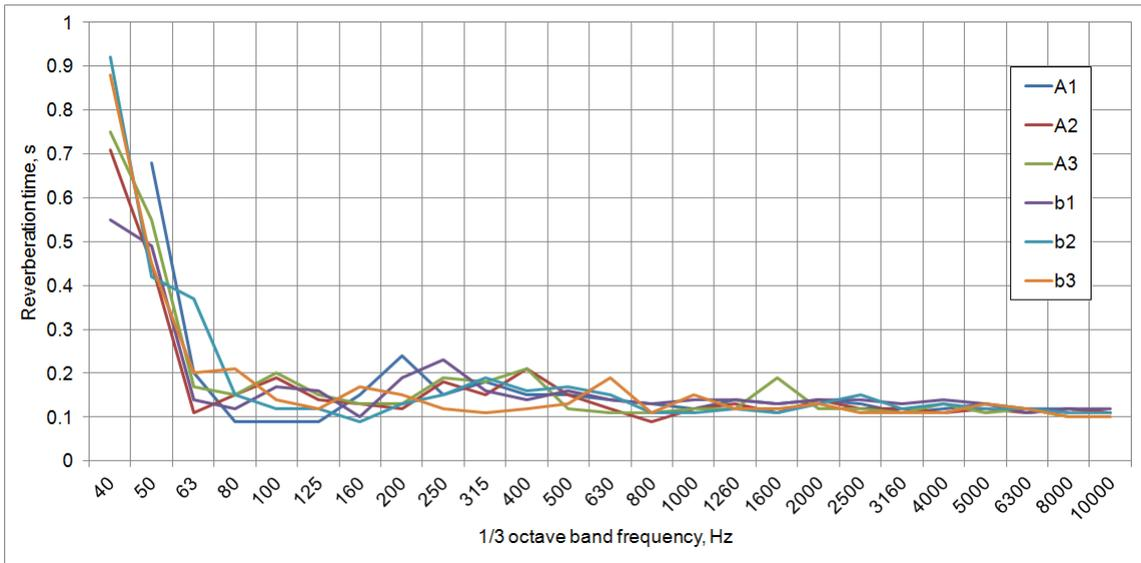
Fig. 2. Results reverberation time measurements in the acoustic chamber (A1 – A3 – sound source placed in the center of the chamber, b1 – b3 – sound source placed in the corner of the chamber).
