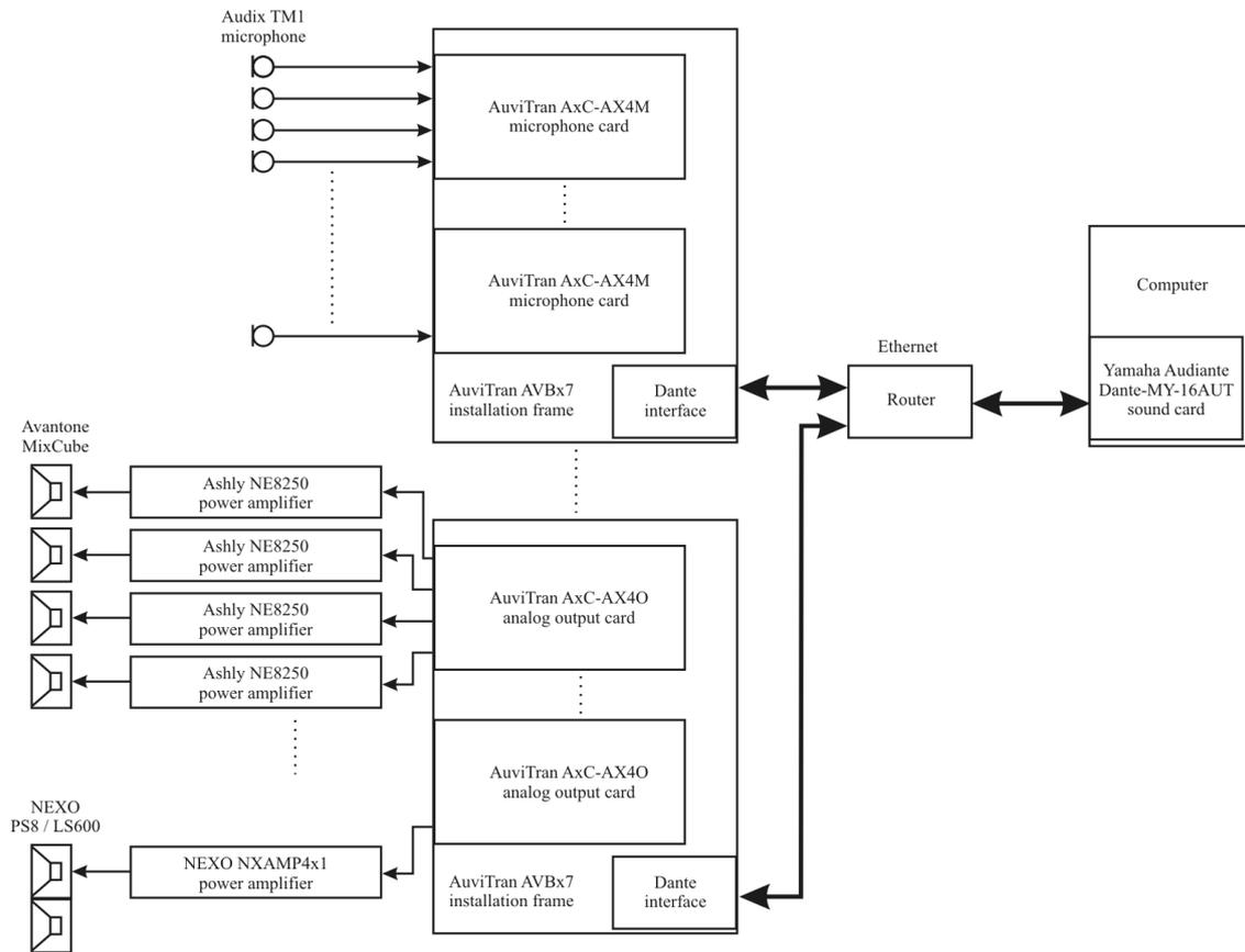
Fig. 4. Schematic diagram of the multichannel sound reproduction and recording system.
