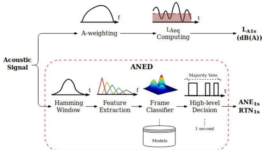
Figure 4: ANED diagram.
