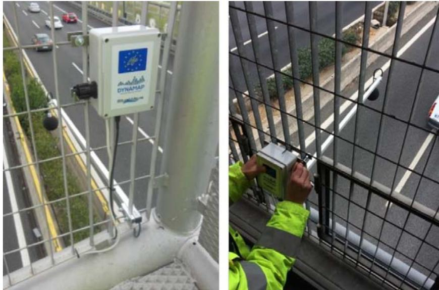
Figure 3: View of the Hi-Cap sensor installed in a portal of the A90 motorway in Rome
