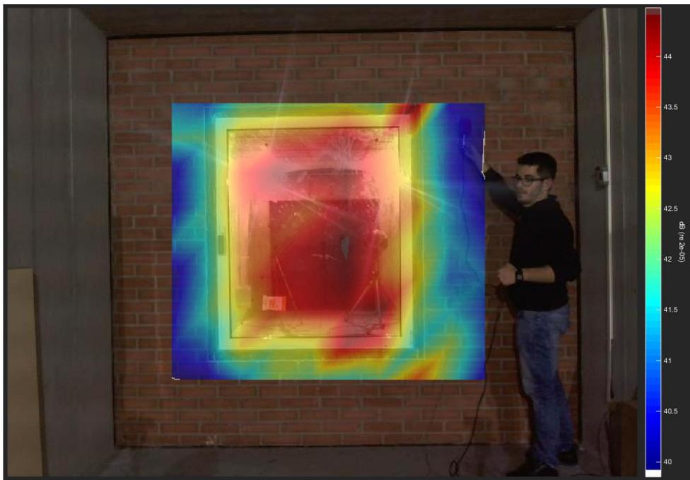
Figure 5 - Averaged Sound Pressure 3000Hz-5000Hz
