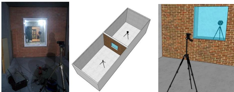
Figure 1 - Scanning measurement setup
