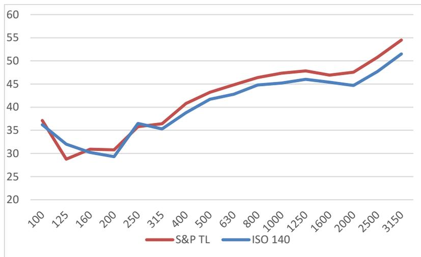
Figure 10 - Comparison of Sound Transmission Loss results
