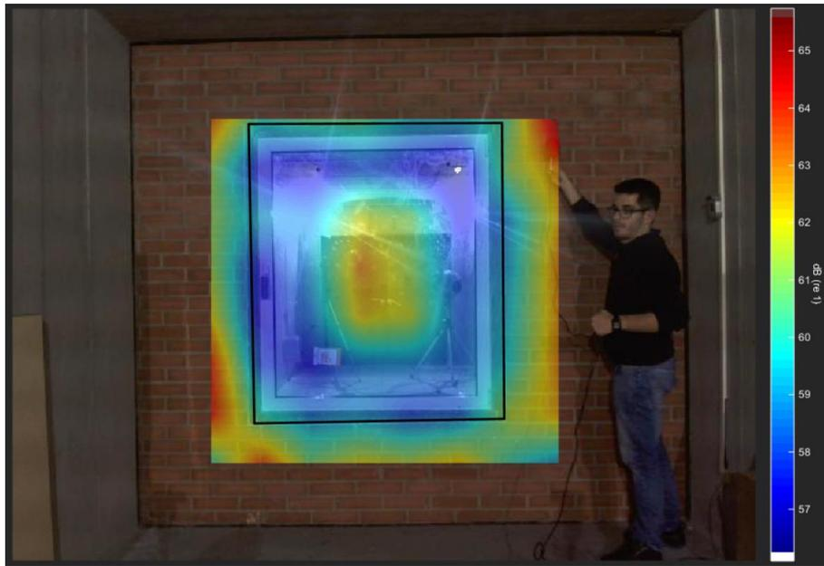
Figure 9 - Transmission Loss in 4000Hz band
