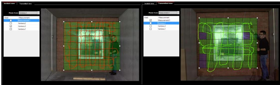
Figure 6 - Grid configuration for TL calculations
