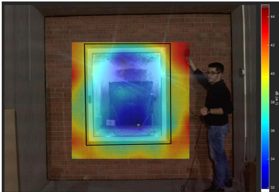
Figure 8 - Averaged Transmission Loss 100Hz-3150Hz
