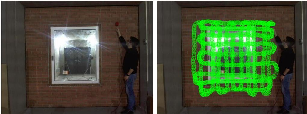
Figure 2 - Receiver room scanning
