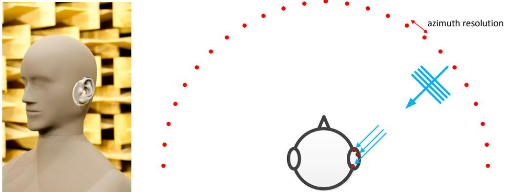
Figure 3: Definition and measurement of the multichannel-HRTF at the positions of the hearing aid's microphone
