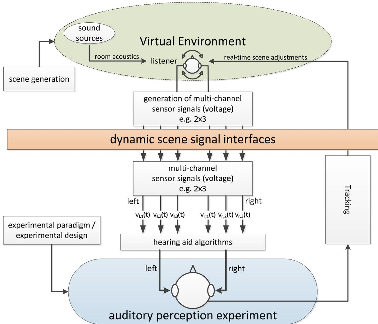
Figure 1: Concept of a dynamic acoustic room simulation for hearing aids with binaural technology
