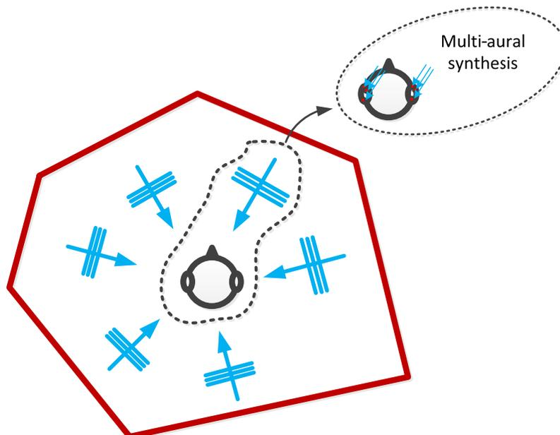
Figure 4: Virtual environment of a complex acoustic situation (red). Multichannel synthesis by means of plane wave fields and convolution of the respective simulated paths with direction depending multichannel HRTF (cf. Figure 3)
