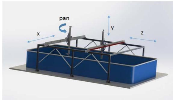
Fig.2. Cad design of calibration tank installed at laboratory facilities of Unidad Mixta IEO-UPV located in Gandia's harbour.
