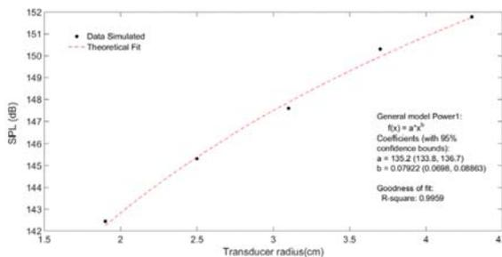
Fig.7. Expected relation of sound pressure level amplitude for difference frequency parametric beam with radius of transducer.
