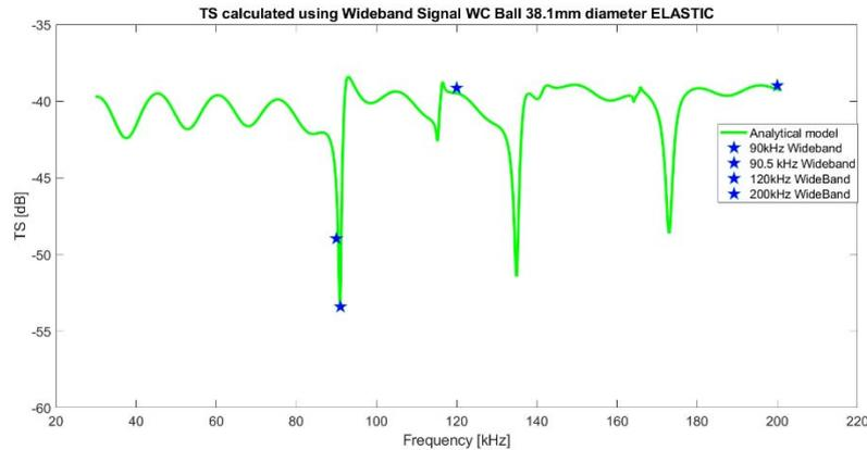
Fig.11. This figure contains results obtained considering fluid-solid interaction. In this case only wide band signals has been used to calculate TS.
