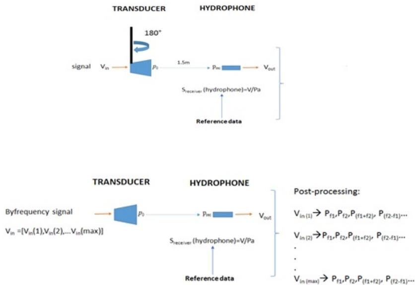
Fig.3. Detail of type of measurements performed depending on signal used to feed the prototype transducers. Directivity of beams were measured using the pan axis rotation applied on the emitter. Distance among emitter and receiver was 1.5m.
