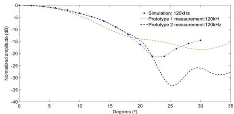
Fig.4. Experimental and simulated directivity considering transducer prototype 1 and prototype 2, for linear case signal of 120kHz.
