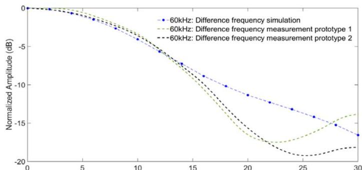
Fig.5. Experimental and simulated directivity considering transducer prototype 1 and prototype 2, for non linear case, parametric beam of 60kHz.
