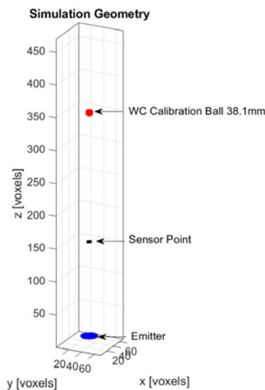
Fig.8. Detail of simulation scheme developed in kwave toolbox
