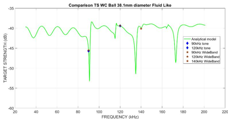
Fig.10. Comparison among TS calculation results considering wideband signal, tone signals at required frequencies and analytical model assumed as a accepted as an accurate result. Results obtained corresponds to fluid like interaction, this means that computation does not consider shear waves propagation and calibration sphere presents only compressional waves.
