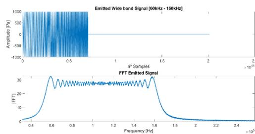
Fig.9. Broadband signal used to calculate de target strength of calibration sphere (Chirp with frequency range from 60kHz to 160kHz)
