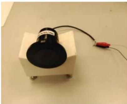
Fig.1. Detail of planar transducer prototype used as a parametric non-linear difference beam generator.
