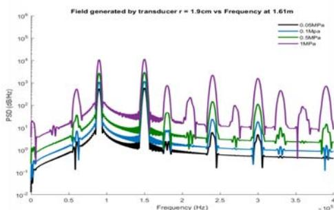
Fig.6. Detail of sound pressure level calculated using kwave, considering different pressure level at vibrating surface.
