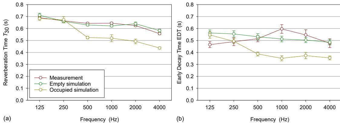
**Figure 8.** Spectral behaviour, spatially averaged, of measured values, and simulated values with the empty theatre, and with 100% occupancy: (a) for  $T_{30}$  parameter, and (b) for EDT parameter. Vertical bars value the spatial dispersion through the standard error.
