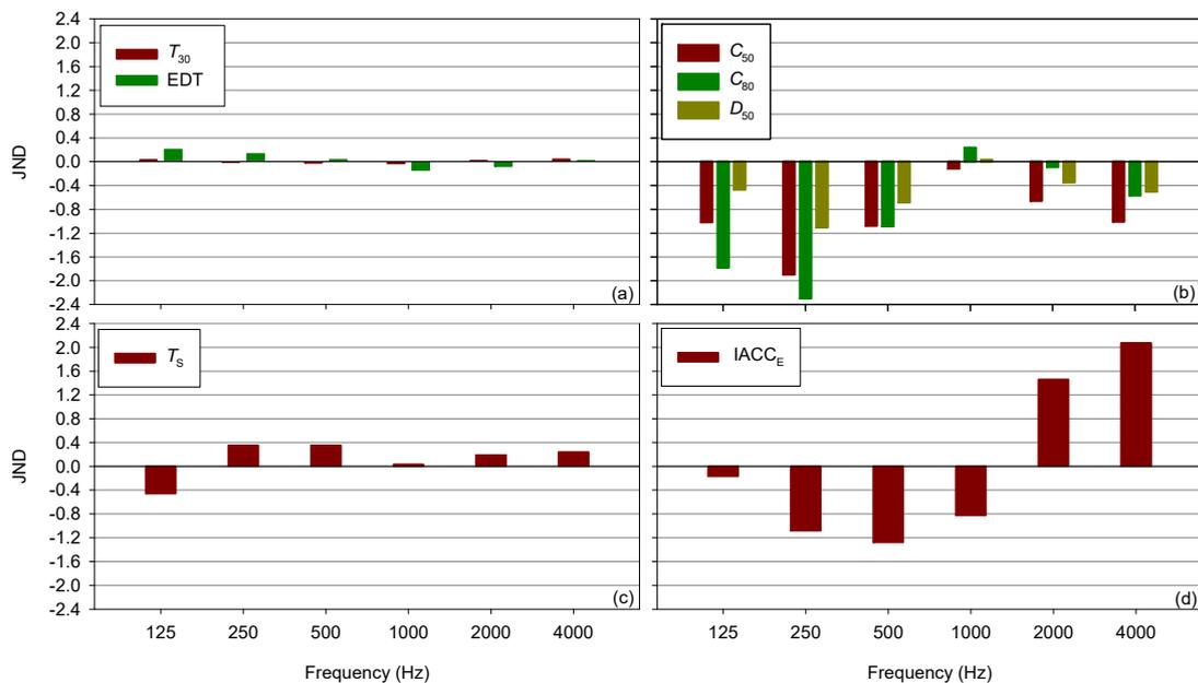
**Figure 7.** Spectral behaviour of the differences between the spatial average of the measured and simulated values of acoustic parameters: (a)  $T_{30}$  and EDT; (b)  $C_{50}$ ,  $C_{80}$  and  $D_{50}$ ; (c)  $T_s$  and (d)  $IACC_E$ .
