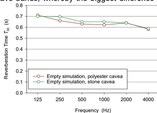
**Figure 9.** Spectral behaviour, spatially averaged, of  $T_{30}$  simulated values with polyester and stone *cavea*.
