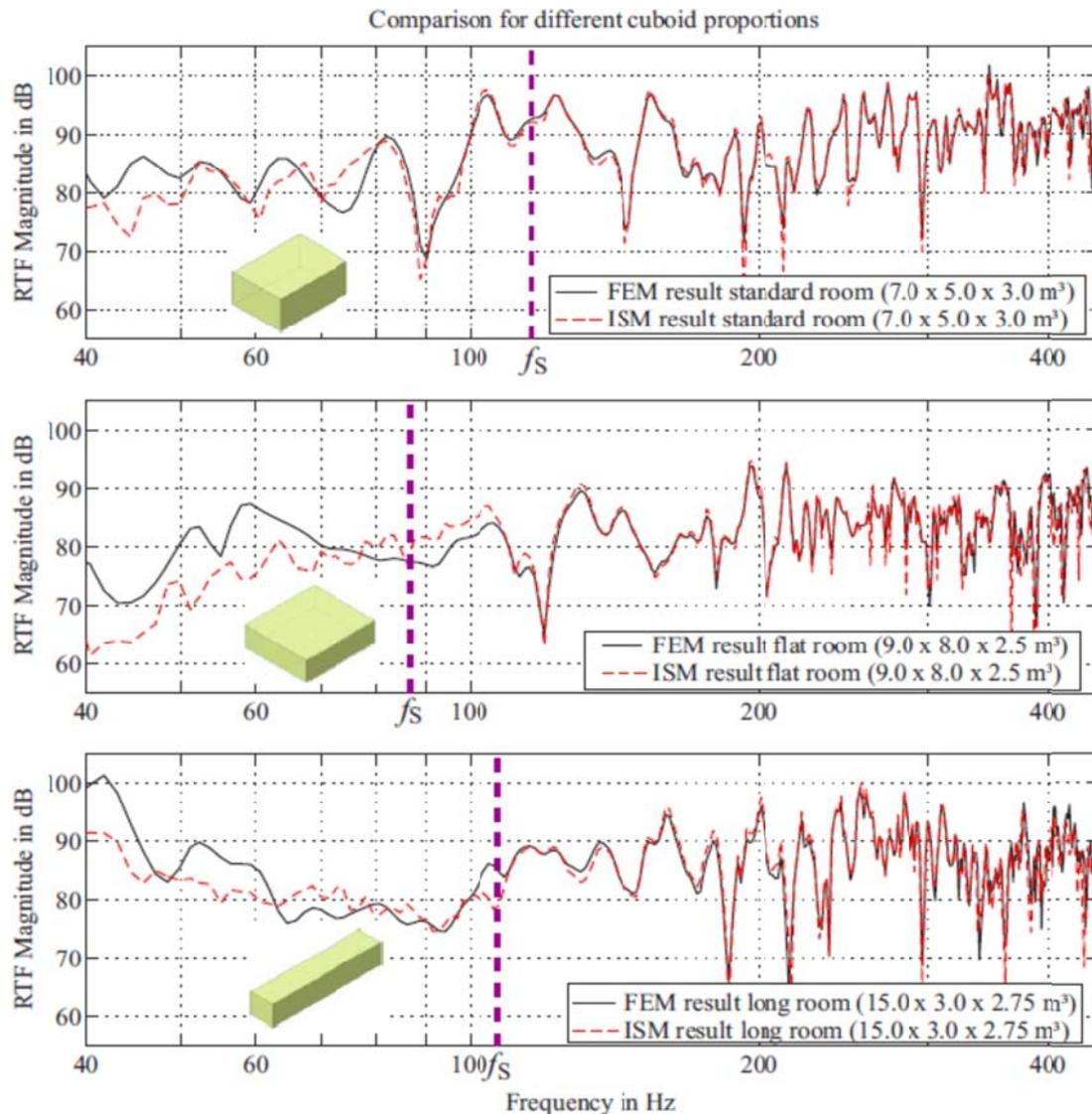
Figure 3. Room transfer functions calculated by using the image source model and FEM [9]
