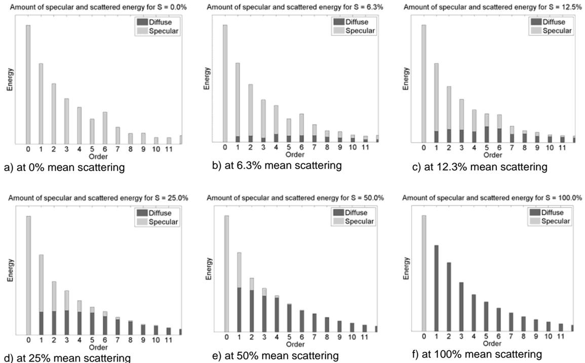
Figure 2. Ray tracing simulations for determination of specular and scattered energy for various mean scattering coefficients.
