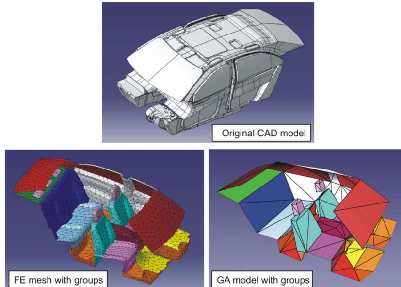
Figure 4. CAD models from car industry and their transformation into acoustic models for the low frequency part (left) and the high frequency part, from [12]
