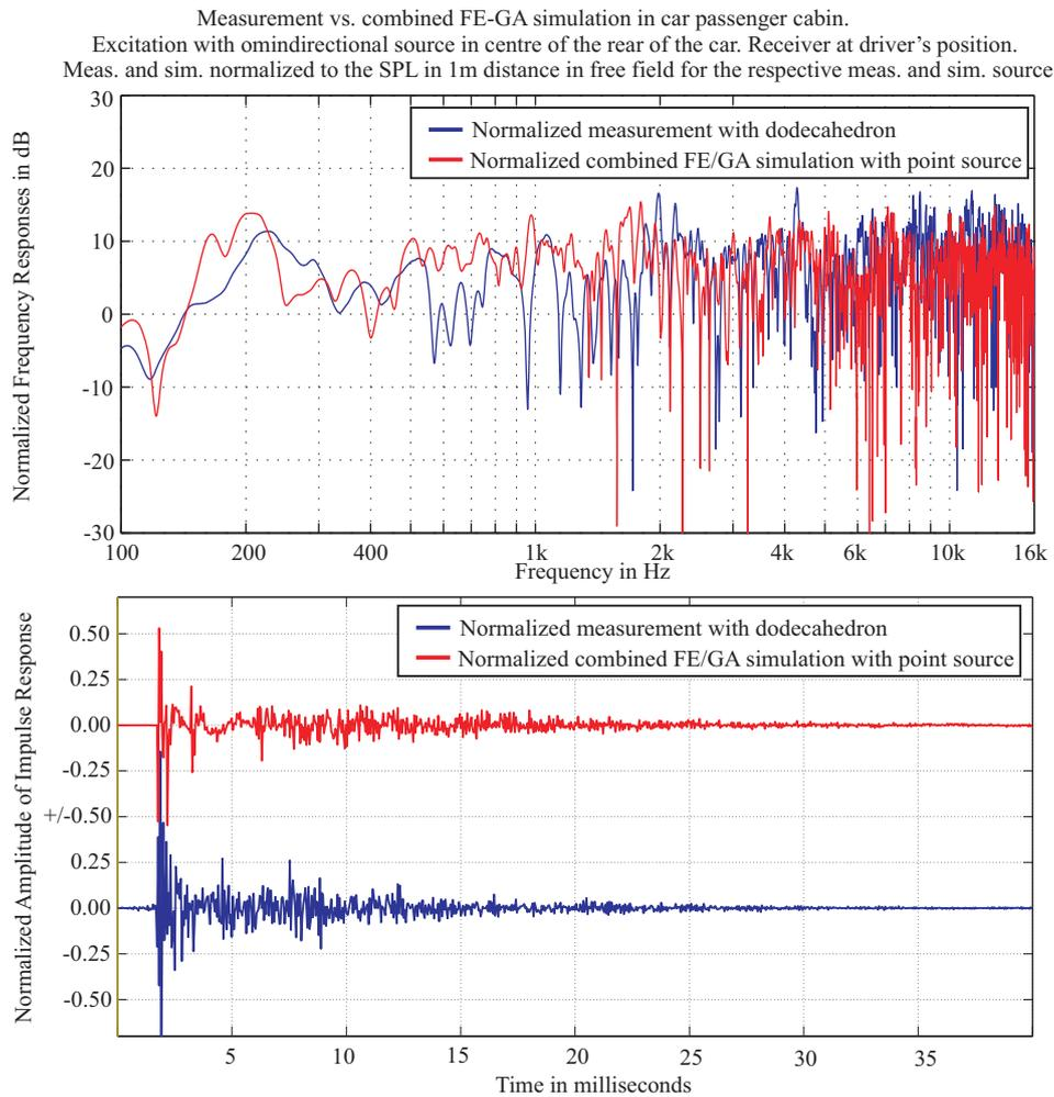
Figure 5. Comparison of simulated and measured frequency response in the passenger cabin, from [12]
