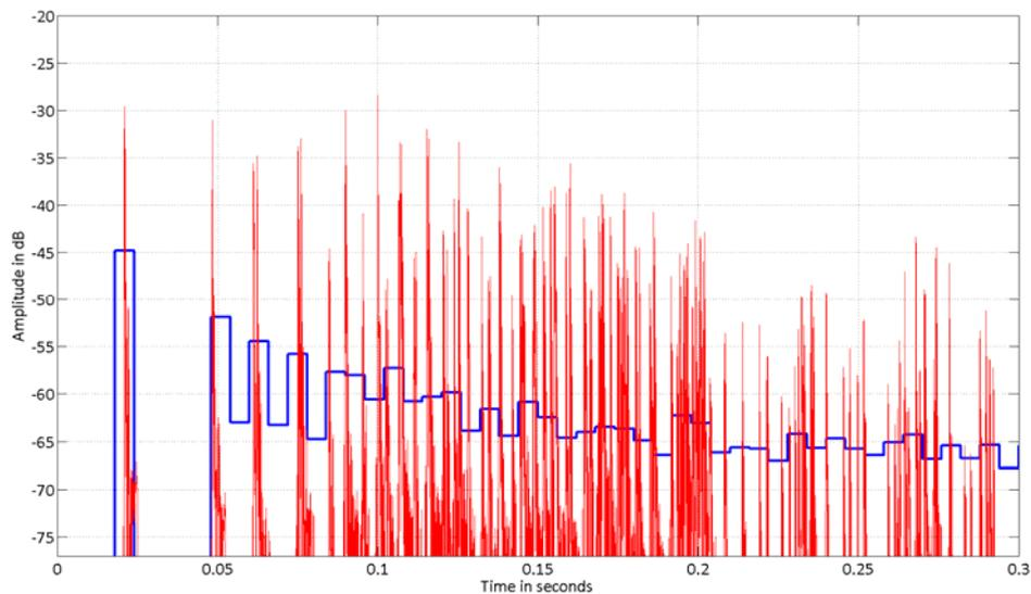
Figure 1. Fundamental energy impulse response computed by using image sources (detailed response) and ray tracing (histogram). (from [4])
