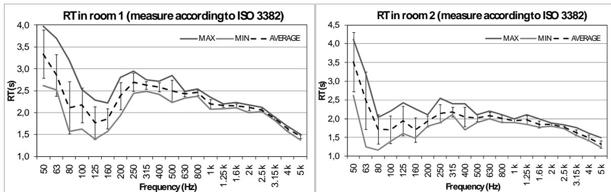
Figure n. 7 – Reverberation time in the two rooms: average of 6 measure points, max and min values.
