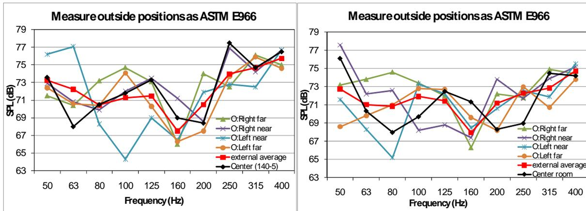
Figure n. 4 – SPL measured in the positions given by the ASTM E 966 for the nearby average method (see fig. 1) in the rooms of fig. 2: room 1 (left) and room 2 (right).
