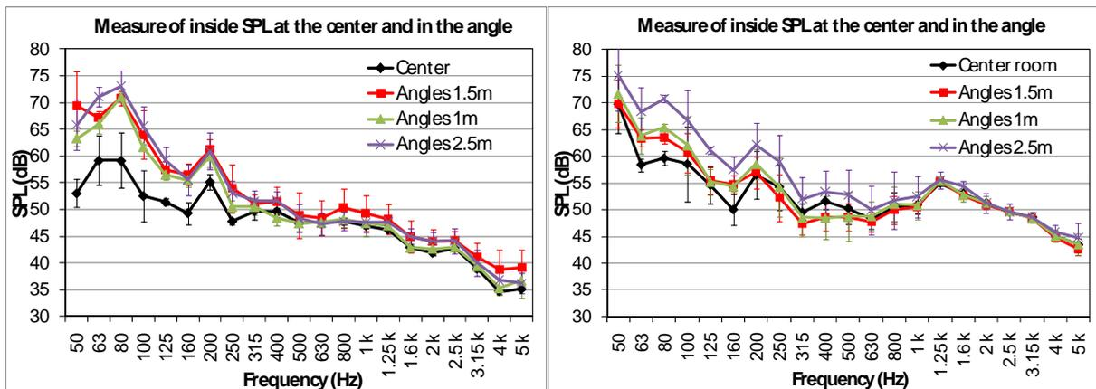
Figure n. 6 – SPL in the corners of the room at different heights (standard deviations refer to the four angles) and average values in the center of the rooms in room 1 (left) and room 2 (right).
