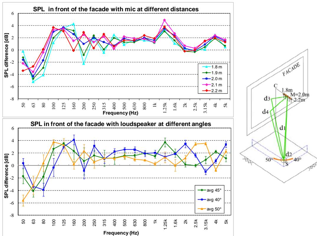
Figure n. 3 – Difference of SPL measurements at 1.8, 1.9, 2.0, 2.1, 2.2 m in front of the façade and at a reference position with the loudspeaker forming an angle of 45° (above) and difference at 2.0 m with the loudspeaker at 40°,45° and 50° (below). Data already reported in Berardi *et al.*, 2011.
