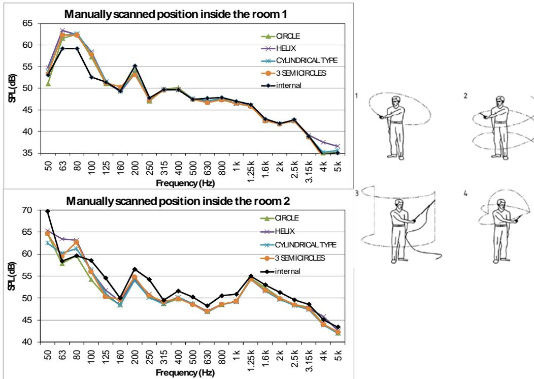
Figure n. 5 – SPL measured through manually-scanned microphone according to the ISO 16283-1, and comparison with the values obtained by average of fixed positions (internal).
