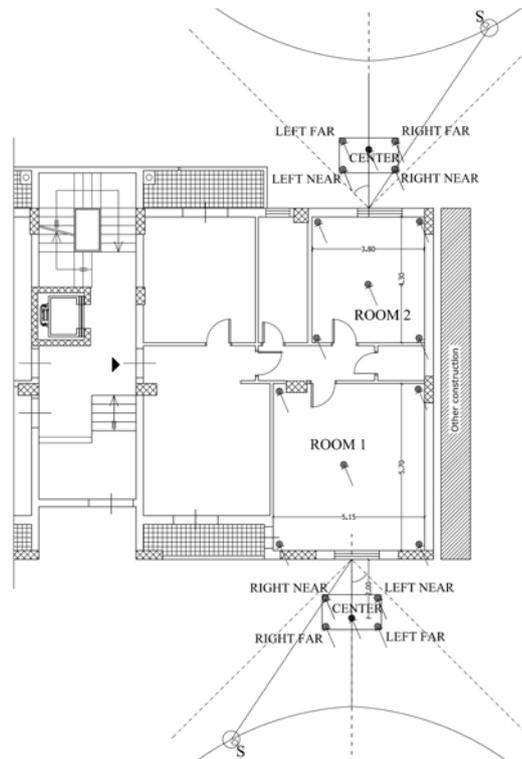
Figure n. 2 – Plan of the building with points of measurement inside and outside the rooms.
