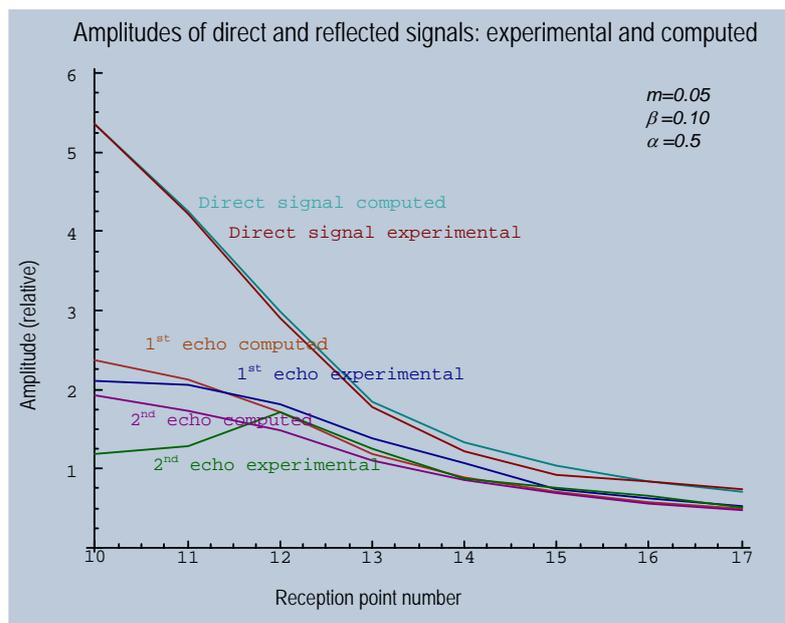
Figure 3.2.2. Global optimization of  $m, \beta$  and  $\alpha$  for the complete signal in experimental study to match simultaneously amplitudes of direct signal and first two echoes
