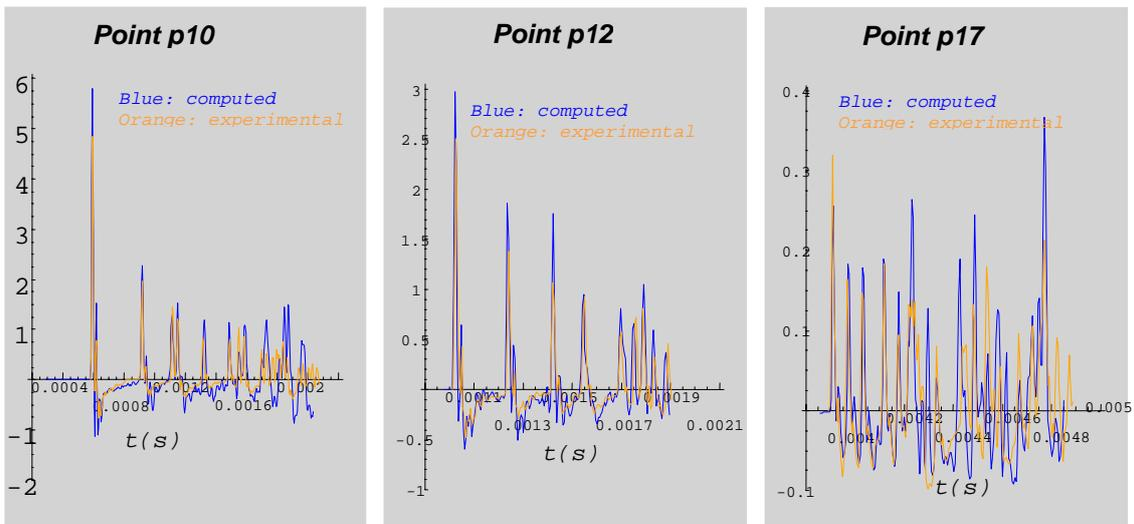
Figure 3.4.1. Comparison of experimental and computed echograms in points p10, p12 and p17 for the complete signal.
