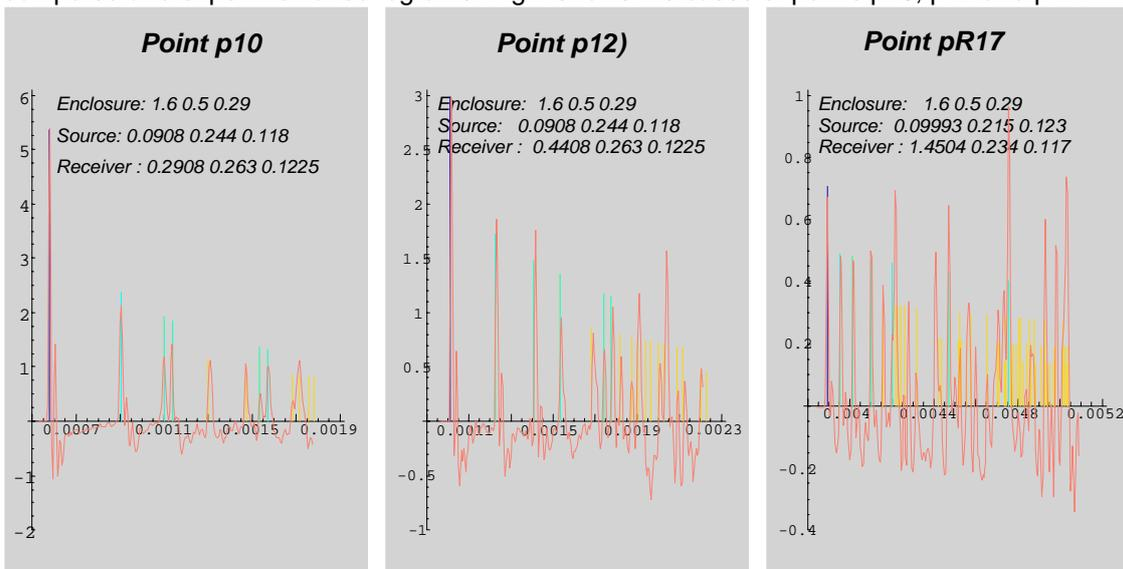
Figure 1. Matching arrival times of computed image sources (blue: direct; green: first order; yellow: second and higher orders) to experimental echograms (red)
