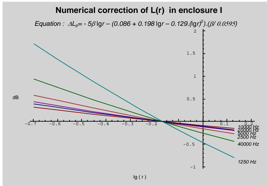
Figure 3.5.1. Differences on sound level as a function of distance in rectangular enclosures
