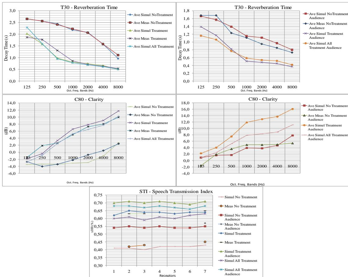
Figure 6 – Comparative results of the analysis covered by this study for the situation of without an audience and with an audience, except for the STI analysis. (i) *Treatment* corresponds to the adopted acoustical treatment solution and (ii) *All Treatment* corresponds to treatment material on all the area of the ceiling (simulation only).
