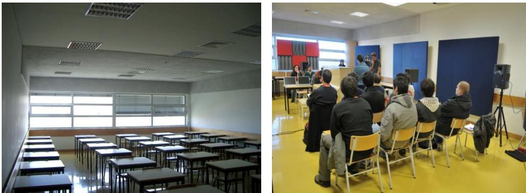
Figure 4 – Photograph view of the room C3.16 and C3.14 with acoustical treatment applied (gray color). Room C3.14 with supplemental acoustical treatment based on absorbed and diffusers panels (right).
