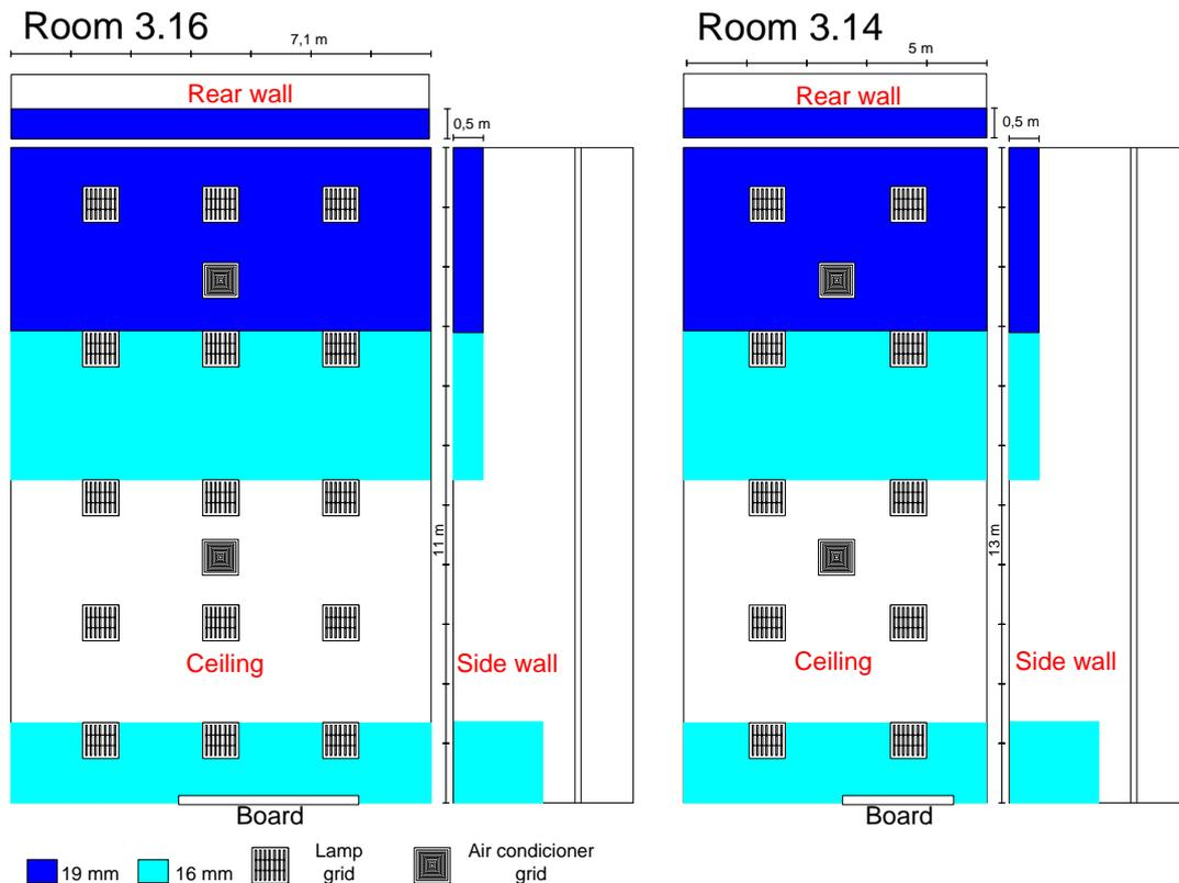
Figure 3 – Location of the acoustical treated areas, walls and ceiling, showing the different thickness of the material.
