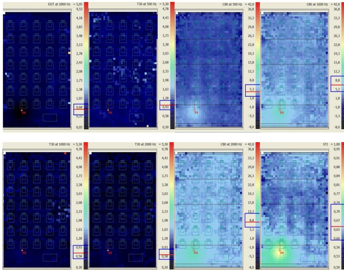
Figure 7 –Results of the analyses of the acoustical parameters for all the area of the audience with renovated room. Placed on the color scale, on the right side of each figure, are the bounds for each parameter (blue color). The lower value indicates that only 5% of the grid results are below, and the upper value assures that more than 95% of the grid results are below. The red segment shows the average value.
