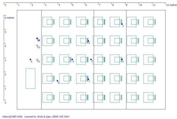
Figure 1 – Classroom C3.16 with the measurement points.
