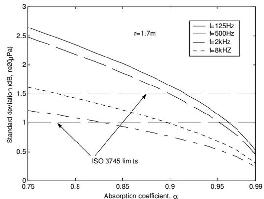
Figure 4 – STD as a function of wall average absorption coefficient at several frequencies.
