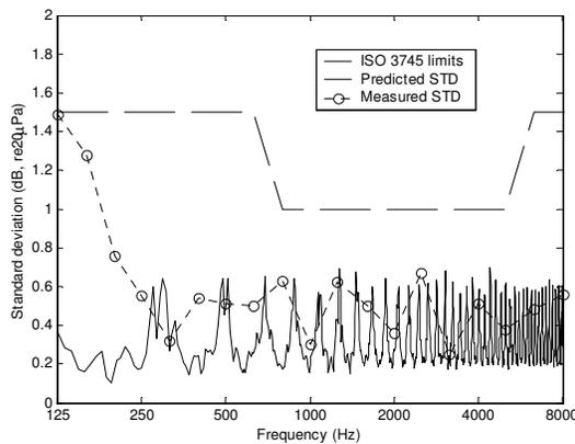
Figure 3 - STD as a function of frequency at 1.4m from test source.
