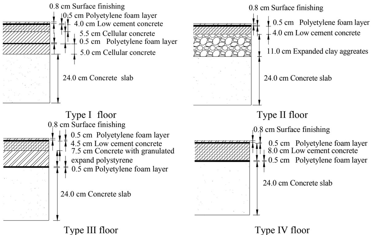
Figure 2 - Schematic section of the floors
