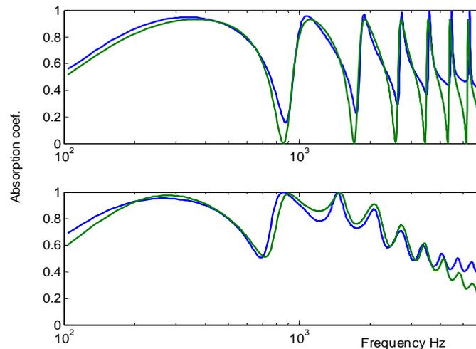
Figure 3. Absorption spectra of the combination perforated panel and absorptive material. Air cavity 20 cm.
