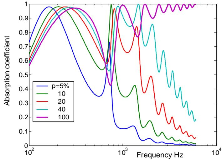
Figure 5 Absorption versus plate perforation coefficient. Panel thickness  $t=11$  mm
