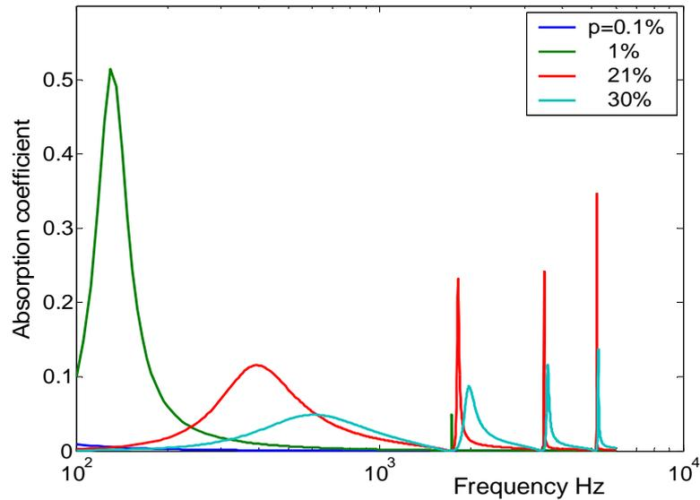
Figure 1 Absorption coefficient in function of the perforation coefficient
