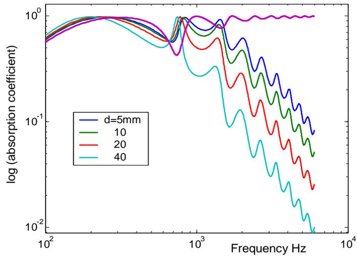
Figure 6 Absorption versus holes diameter. Perforation ratio  $p=23\%$ ,  $t=11$  mm.
