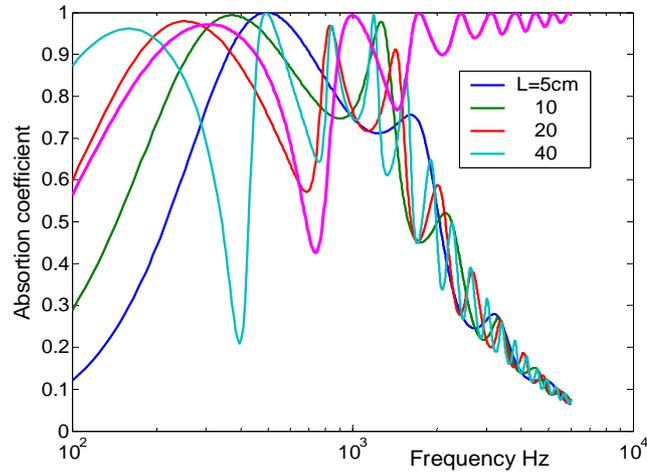
Figure 7 Absorption versus air cavity.  $p=23\%$ ,  $t=11$  mm, hole diameter  $d=6$ mm
