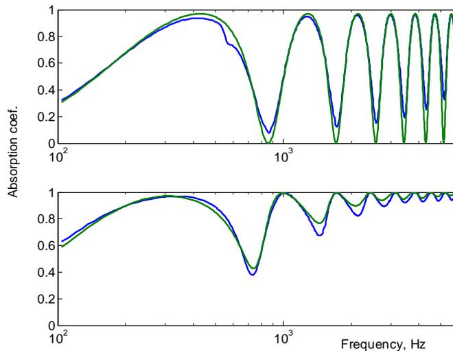
*Figure 2 Acoustic absorption of a 4.5 cm layer of mineral wool (upper), and a non woven textile. Air cavity 20 cm.*
