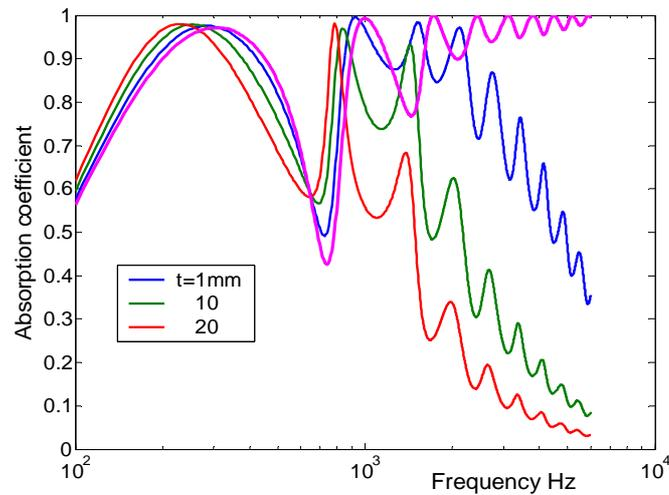
Figure 8 Absorption versus panel thickness. Perforation coefficient  $p=23\%$ , Air cavity 20 cm. Magenta: absorption without perforation panel
