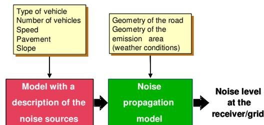
Figure 1- The distinction between noise sources and propagation
