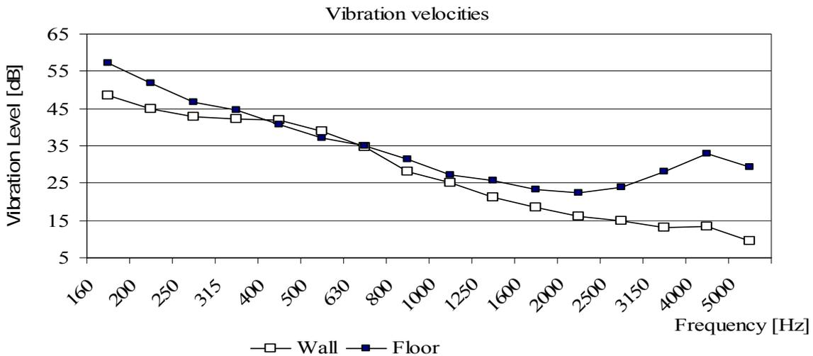
Figure 4 – Vibrations velocities for floor and wall
