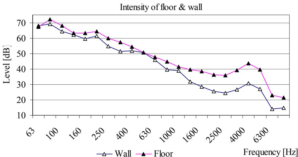
Figure 3 – Intensity measurements of floor and wall
