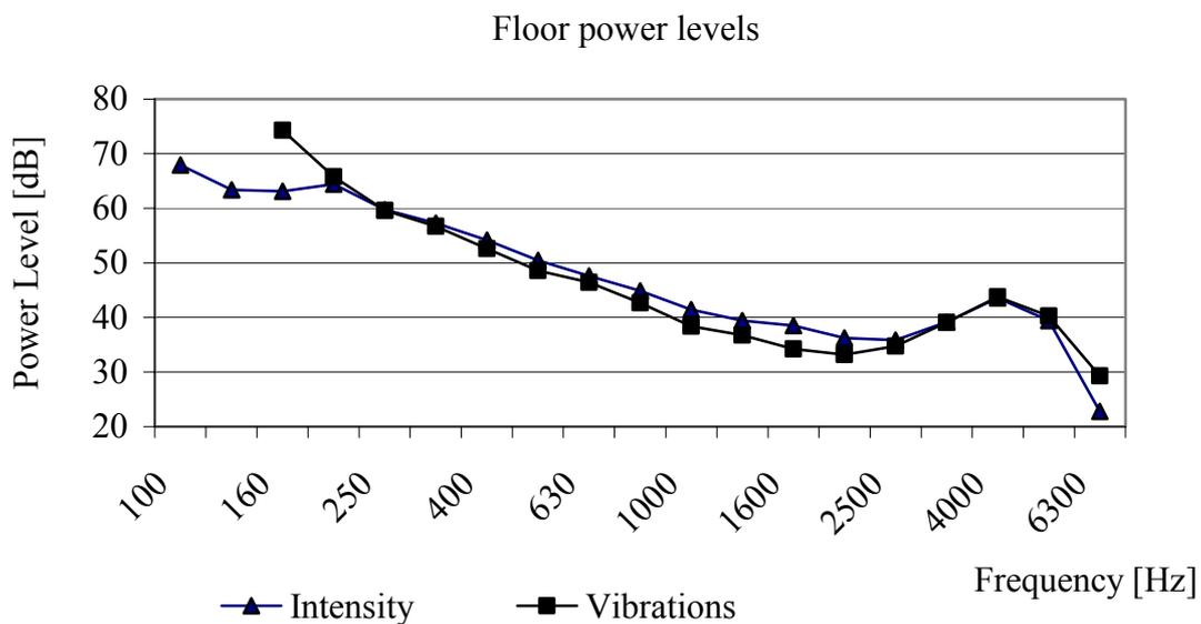
Figure 5 – Compared results for the floor
