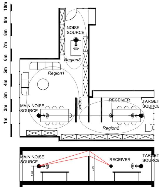
Figure 1 - Ground floor and section of the room (ceiling height is 2.7 m)
