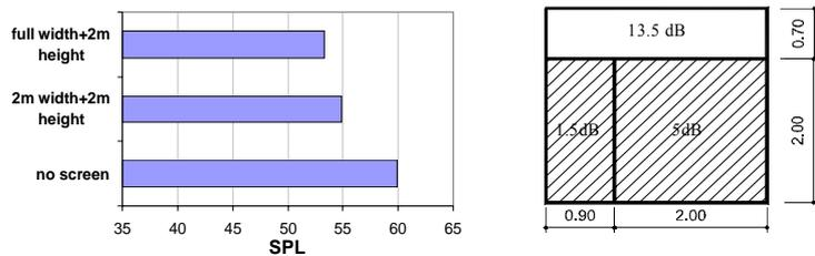
Figure 5 - Effect of screen width and graphical representation of the screen and SPL decreases caused by each piece.
