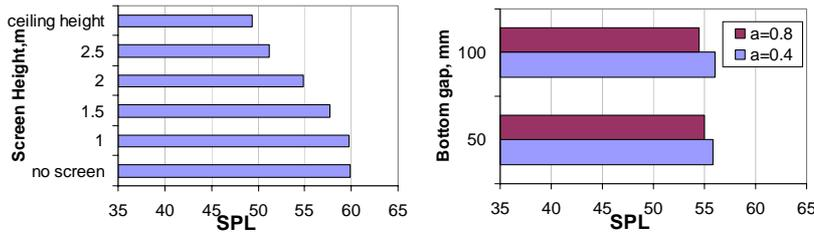
Figure 3 - Effect of screen height on SPL and effect of bottom gaps (2x2 m screen)
