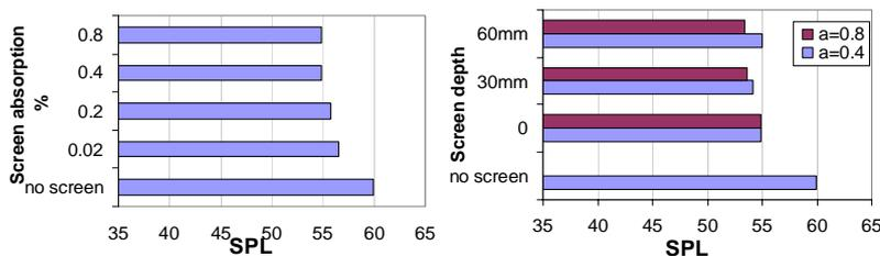
Figure 4 - Effect of absorption on screen and effect of depth (2x2 m screen)
