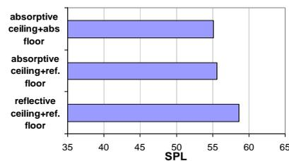
Figure 6 - Effect of absorptive ceiling and floor (2x2 m screen)
