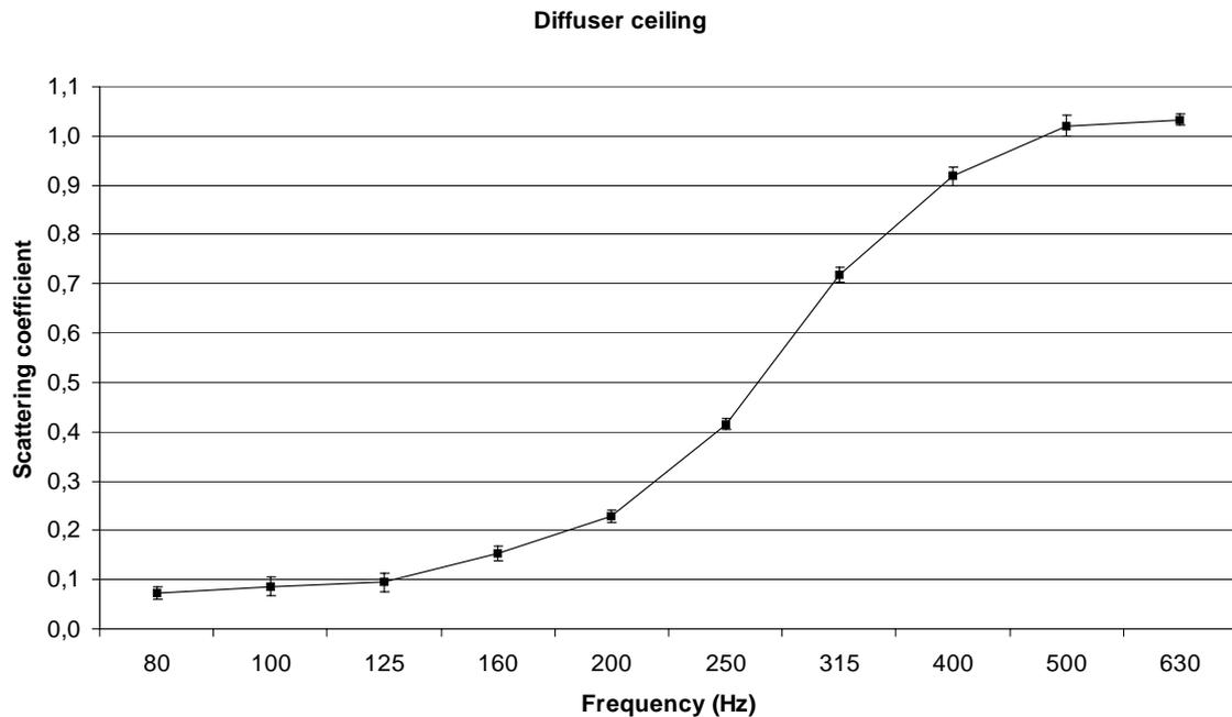
Figure 3 – Measured random-incidence scattering coefficients of the diffuser on the ceiling of the studio at the PTB. The results are shown as a function of the full-scale frequency.
