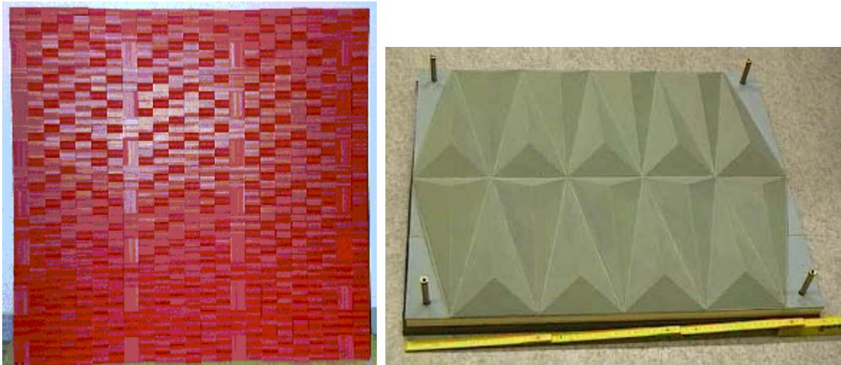
Figure 1 – Samples from the wall (left) and ceiling diffuser (right) of the studio at the PTB. Picture at the right taken from [www.ptb.de/en/org/1/17/173/roundrob3\\_2.htm](http://www.ptb.de/en/org/1/17/173/roundrob3_2.htm).
