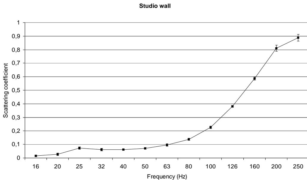
Figure 2 – Measured random-incidence scattering coefficients of the diffuser on the wall of the studio at the PTB. The results are shown as a function of the full-scale frequency.
