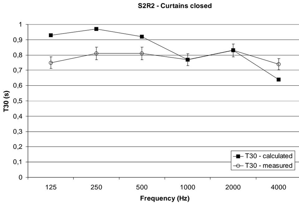
Figure 5 – Reverberation Time measured and simulated at position S2R2, with curtains closed. The error bars indicate the room acoustical subjective limens for this parameter.
