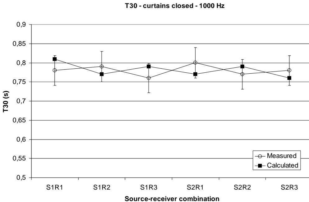
Figure 6 – Reverberation time ( $T_{30}$ ), measured and calculated for all source-position combinations at 1000 Hz, with the curtains closed. The error bars indicate the room acoustical subjective limens for this parameter.
