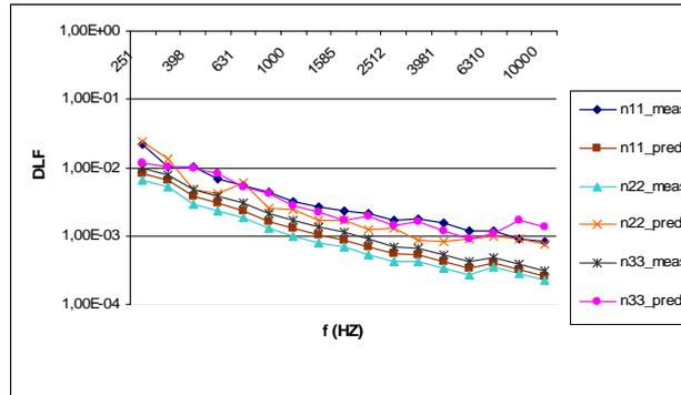
Figure 1 – Comparison between measured and predicted values for the DLF.
