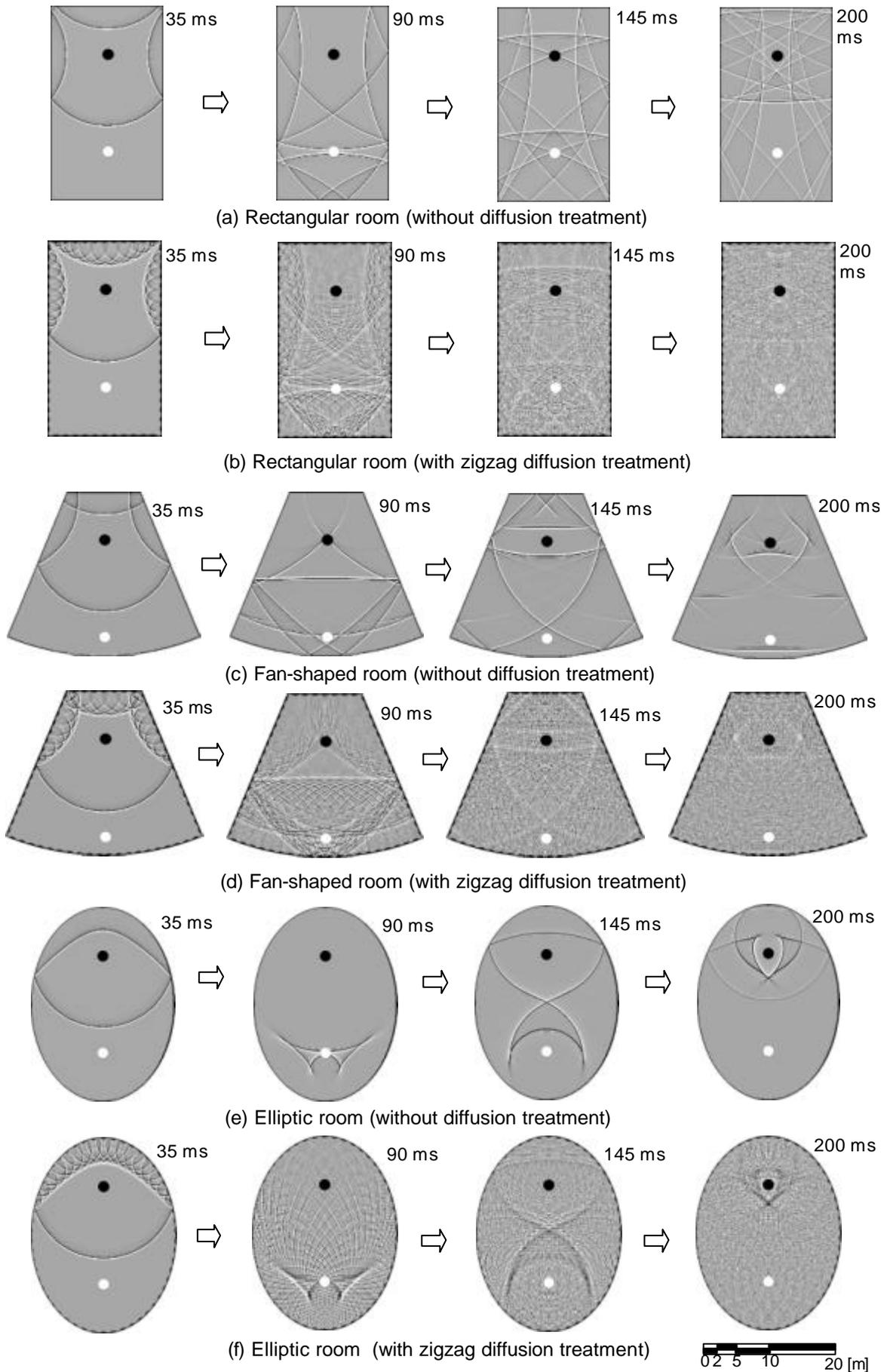
Fig.1 Sound propagation in a rectangular, fan-shaped and elliptic rooms with/without diffusing treatment.
