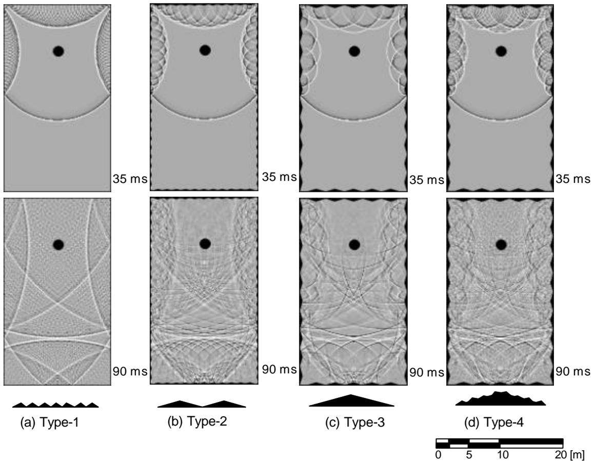
Fig.3 Comparison of sound propagation in the rectangular room with four types of diffusing treatments
