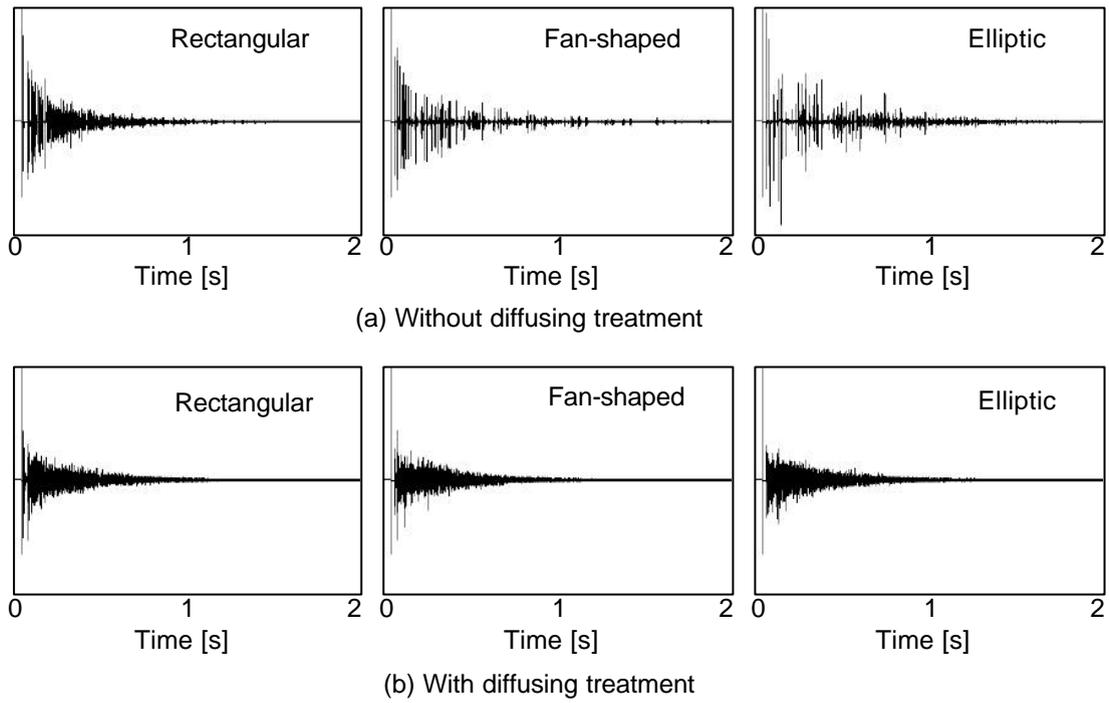
Fig.2 Impulse responses at the receiving points shown in Fig.1.
