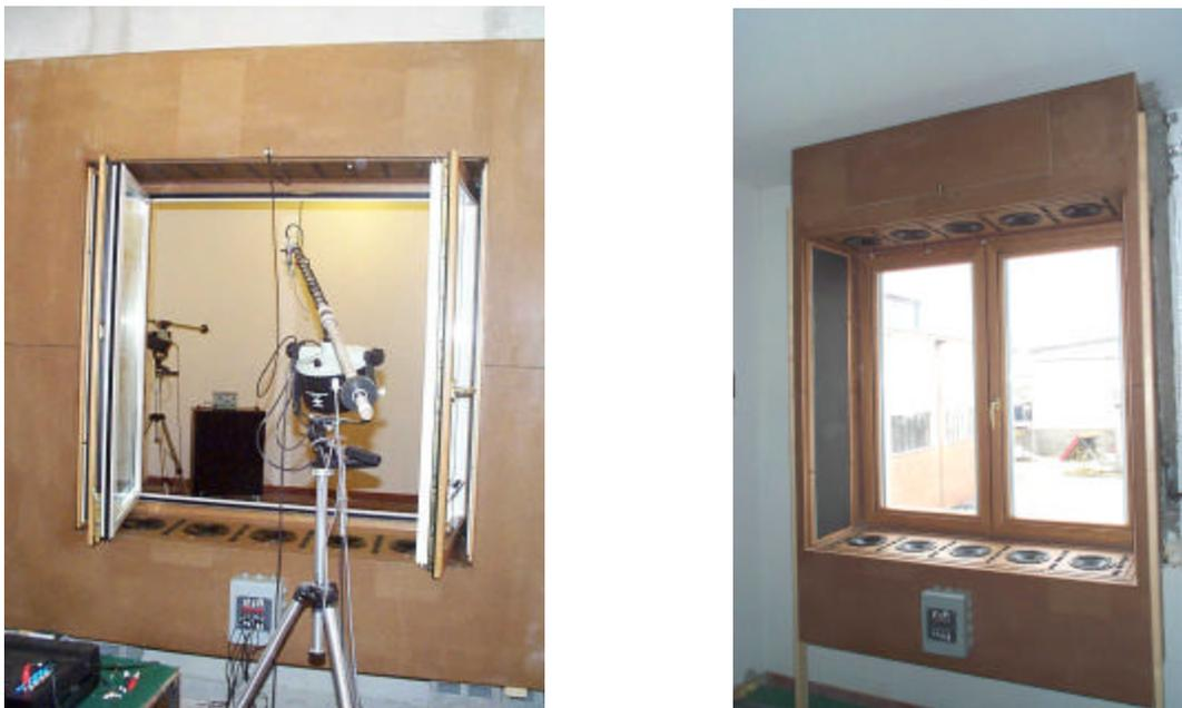
Fig. 2 – Active window: in laboratory (left) and in the experimental building (right).
