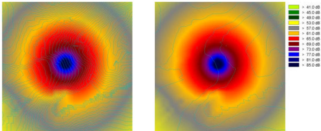
Figure 1. Two noise maps of the same site with a 120 dB point source each and a different number of contour lines per unit area.
