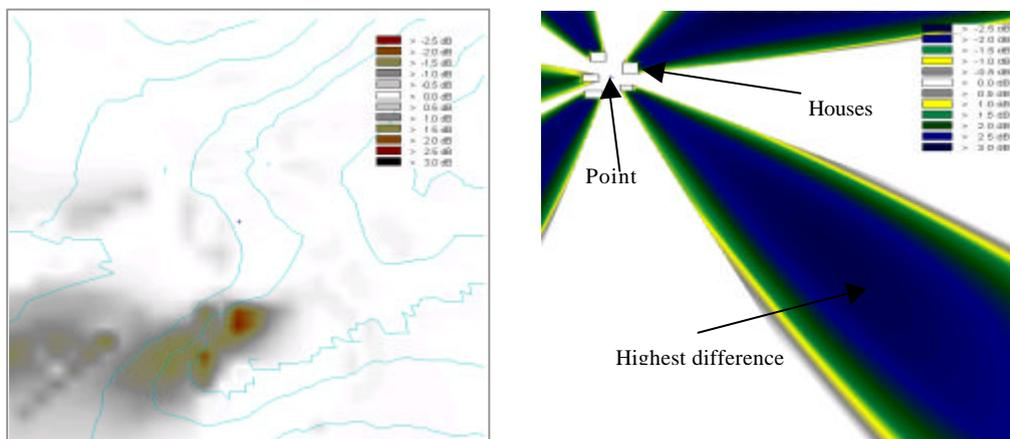
Figure 2. Left: Difference map obtained as the difference between both maps from figure 1. Right: Difference map between 4m and 3m height houses for a fixed 80 dB point source at 1m from the ground. The 2.5 dB difference extends to about 500 m from the source.
