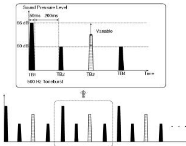
Fig. 1 Time pattern of tone burst sequence used in the experiment
