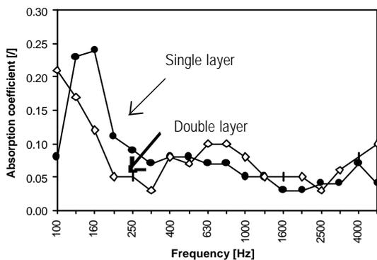
Figure 3 – Comparison between single and double layer configuration
