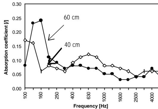
Figure 4 – Comparison between configurations with different studs pitch (60 and 40 cm)
