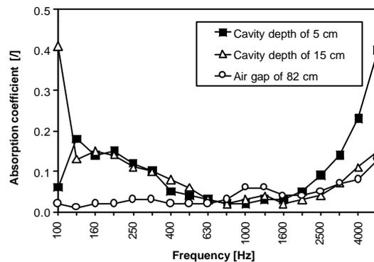
Figure 8 – Absorption coefficients for configurations with plates laid on rectangular frame and different cavity depths
