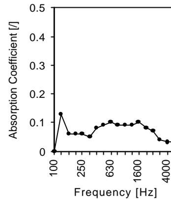
Figure 10: Absorption coefficients of the sample of suspended ceiling tested in the reverberation room
