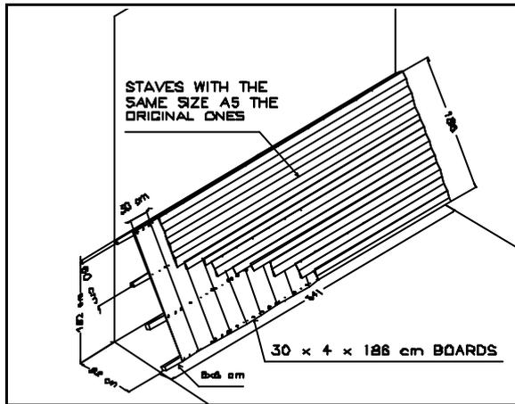
Figure 9: Mounting of the sample in the reverberation room
