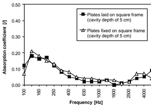
Figure 7 – Absorption coefficients for configurations with different type of connections to the frame
