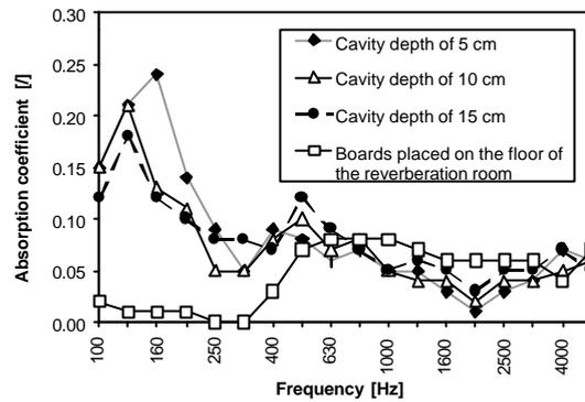
Figure 2 – Absorption coefficients for configurations with single layer of gypsum boards and different cavity depths
