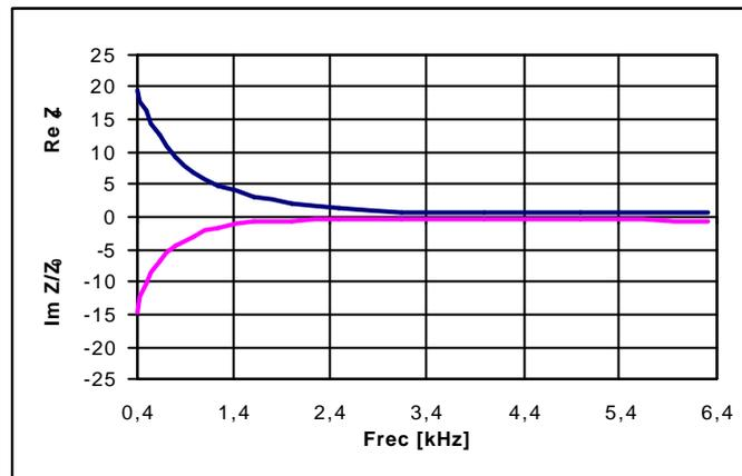
Figure 2 Real and Imaginary parts of impedance ratio for sample 2 of commercial foam.
