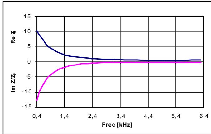
Figure 1 Real and Imaginary parts of impedance ratio for sample 1 of commercial foam.
