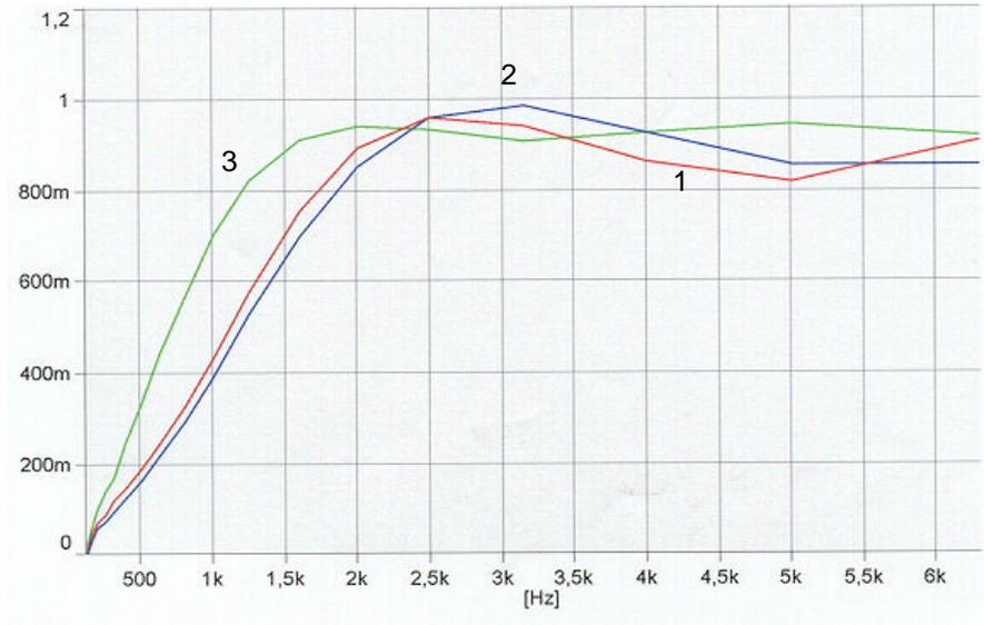
Figure 4. Absorption coefficient for the three samples of commercial foam rubber studied versus frequency in  $1/3$  octave. Red curve 1 corresponds to sample 1, blue curve 2 to sample 2 and green curve 3 to sample 3. See Table I for details.
