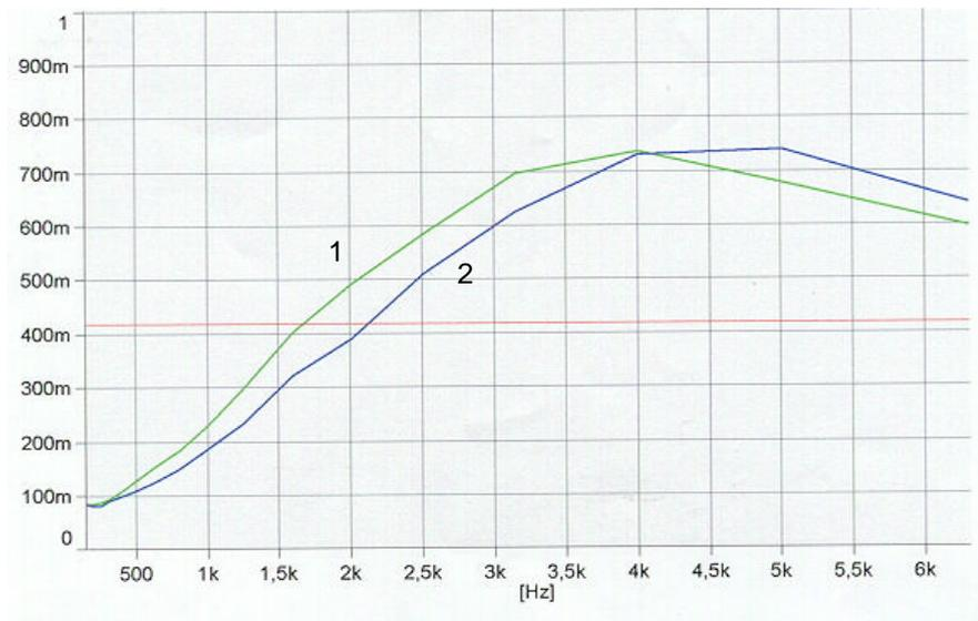
Figure 5. Absorption coefficient for the two samples of bulk foam rubber studied versus frequency in  $1/3$  octave. Green curve 1 corresponds to sample 1 and blue curve 2 to sample 2. See Table I for details.
