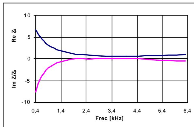
Figure 3 Real and Imaginary parts of impedance ratio for sample 3 of commercial foam.
