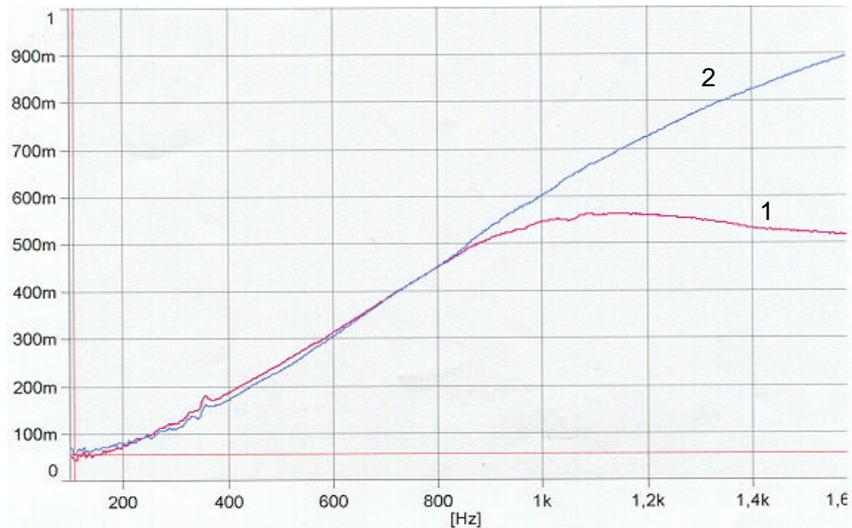
Fig. 6. Absorption coefficient of covered sample (blue curve 1) and manufactured material (red curve 2) versus frequency. See text for details.
