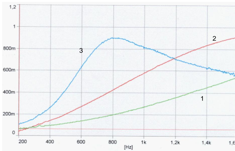
Figure 5. Normal absorption coefficient of the textile agglomerate 1 (green curve 1), that sample with the first resonator (red curve 2) and with the second resonator (blue curve 3). See text for details.
