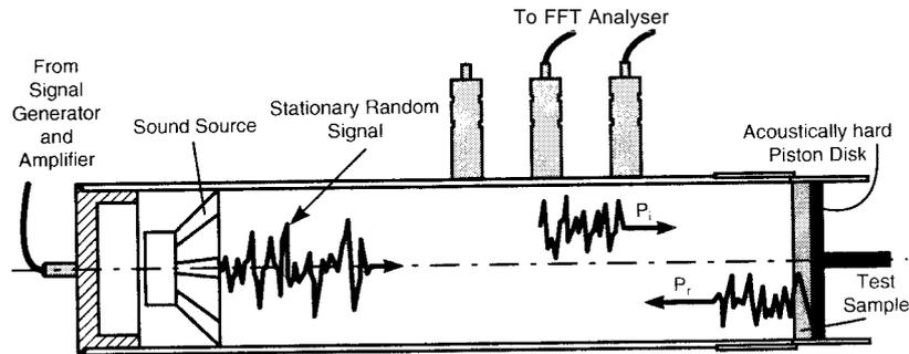
Figure 1: Experimental equipment used to measure the normal absorption coefficient.
