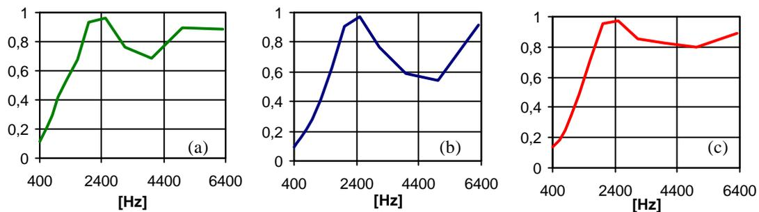
Figure 2. Normal absorption coefficient of metal shaving conformer samples 1 (a), 2 (b) and 3 (c) versus the frequency in  $1/3$  octave.
