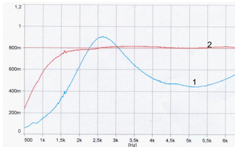
Figure 3. Comparison between the absorption coefficient of the metal shaving conformer (curve 1) and multilayer material (curve 2). See text for details.
