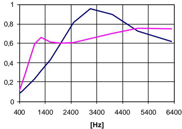
Figure 4. Normal absorption coefficient of textile agglomerate samples 1 (blue curve) and 2 (red curve) versus the frequency in  $1/3$  octave.
