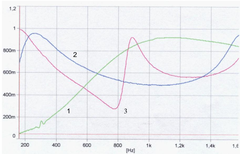
Figure 6. Influence of the air cavity depth behind the sample on the normal absorption coefficient of textile agglomerate 2 with first resonator. Green curve 1 without air cavity behind, blue curve 2 with 100 mm depth of air cavity behind and red curve 3 with double air cavity depth. See text for details.
