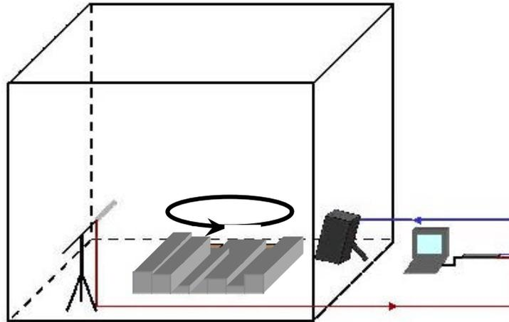
We have obtained the impulse response rotating the diffuser 72 times with a step of 5 degrees. After that, one must perform a phase-locked addition of all the impulse responses obtaining the impulse response for a "virtual" room. (See Figure 4).
