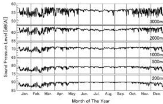
Fig.7. Calculated A-weighted sound pressure levels near the ground of noise generated from an aircraft flying right overhead at heights of 200m ,500m, 1000m, 2000m and 3000m.
