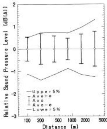
Fig.3. Fluctuation of A-weighted sound pressure levels of noise generated from an aircraft flying near the ground at horizontal distances from 100m to 3200m during a year.
