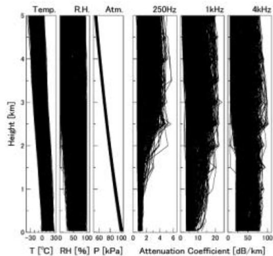
Fig.5. Vertical profiles of air temperature, relative humidity, atmospheric pressure and calculated attenuation coefficients for atmospheric absorption at frequencies of 250kHz, 1kHz and 4kHz during a year.
