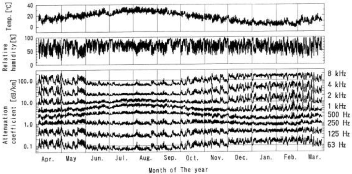
Fig.1. Air temperature, relative humidity and calculated attenuation coefficients for atmospheric absorption at octave band center frequencies form 63Hz to 8kHz during a year.
