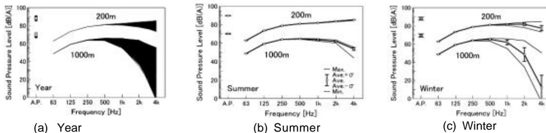
Fig. 8. Calculated sound spectra of noise from an aircraft flying right overhead at heights of 200m and 1000m.
