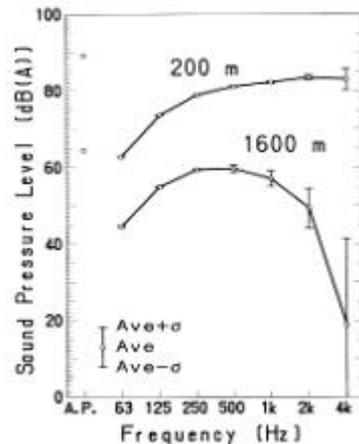
Fig.4. Sound spectra of noise generated from an aircraft flying near the ground at horizontal distances of 200m and 1600m.
