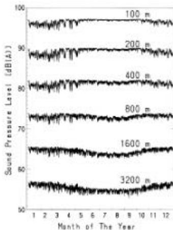
Fig.2. Calculated A-weighted sound pressure levels of noise generated from an aircraft flying near the ground at horizontal distances from 100m to 3200m.
