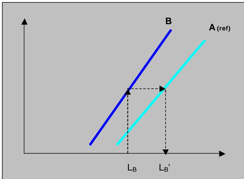
Transformation of a noise from source SB in to an equally annoying noise from the reference source SA
