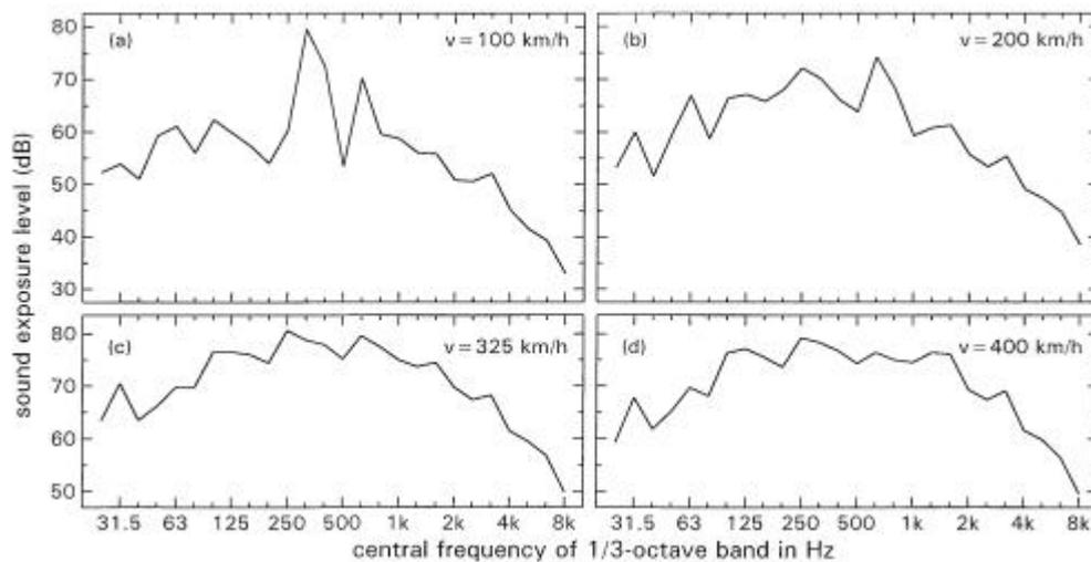
Fig. 1. Spectra determined for four speeds of the Transrapid passbys.
