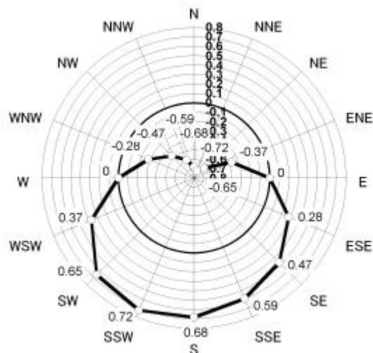
Fig.5. Correlation coefficient of  $U_{vec}$  and  $L_{Aeq,10min,s}$  for each wind-direction
