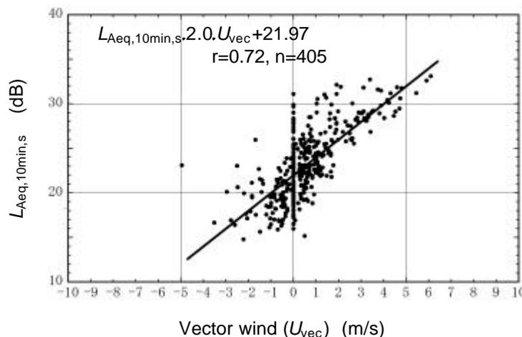
Fig.8 Relation of vector wind ( $U_{vec}$ ) and  $L_{Aeq,10min,s}$
