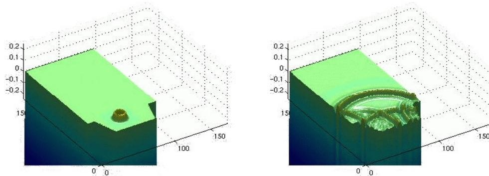
Fig 4. Simulation of a simple stagehouse. On the left the excitation is illustrated. On the right the primary wave front has reached halfway of the hall and diffractions from the edges are visible.
