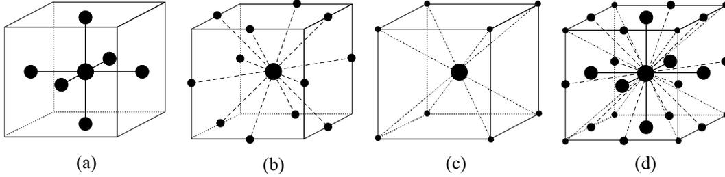
Fig 1. Construction of the interpolated digital waveguide mesh is based on a) the original WGM with 6 neighbors, b) 2-D diagonal neighbors, and c) 3-D diagonal neighbors. Finally, d) the full interpolated WGM structure with 26 neighbors is depicted.
