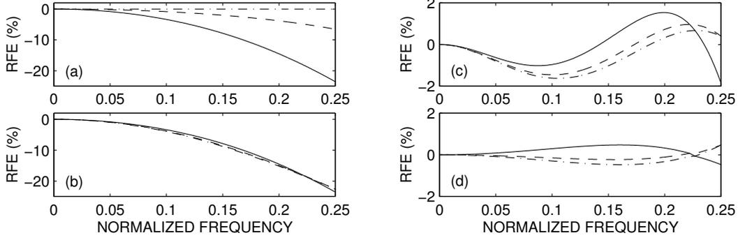
Fig 2. Relative frequency error in the digital waveguide mesh a) in the original structure, b) in the optimally interpolated mesh, c) in the interpolated structure with two-stage multiwarping, and d) in the interpolated mesh with warping in the frequency domain. The curves show RFE in axial (solid line), 2-D diagonal (dashed line), and 3-D diagonal (dash-dotted line) directions. Please note the different vertical scales in left and right columns.
