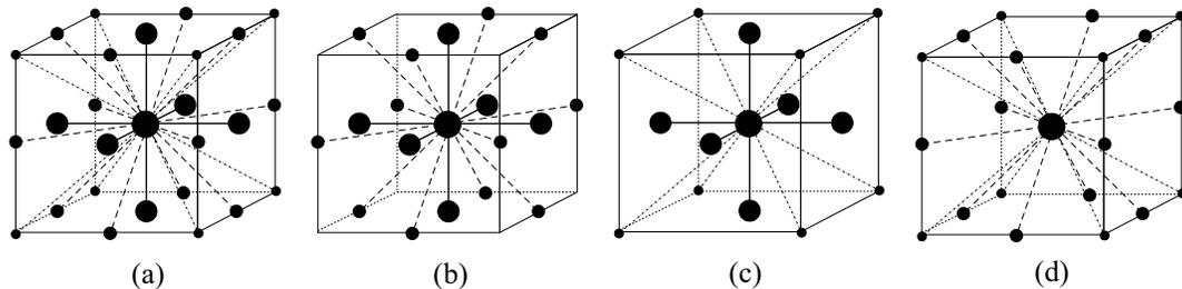
Fig 3. Sparse rectangular mesh structures based on pruning the a) full interpolated WGM structure. In b) the axial and 2-D diagonal neighbors are utilized, in c) axial and 3-D diagonals are effective, and in d) 2-D diagonals and 3-D diagonals are in use.
