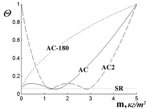
Fig. 5. Efficiency factor for acoustic compensators: single-sided (AC); reversed single-sided (AC-180); double-sided (AC2), and for soft reflectors (SR).
