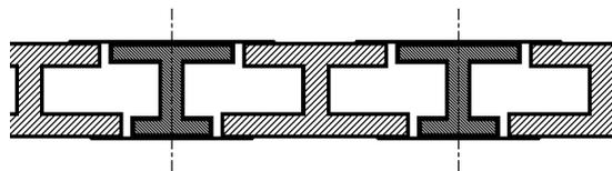
Fig. 2. Double-sided compressible resonators (acoustic compensators).
