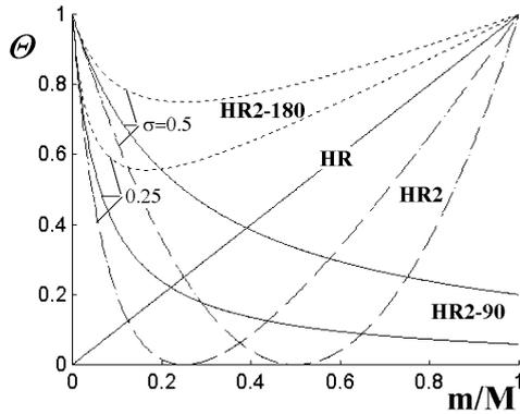
Fig. 4. Efficiency factor of hard reflectors: panel with DVA (HR); straight double-sided hard reflector (HR2); rotated through  $90^\circ$  (HR2-90); turned over (HR2-180).
