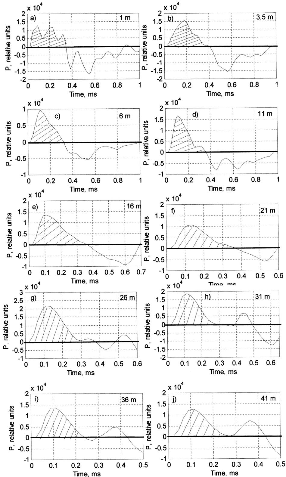
**Fig. 2.** Dependence of the amplitude and form of direct sound of an unfiltered signal upon the distance to the sound source. a), b), c), d), e), f), g), h), i), j) – distance from the microphone to the sound source is equal to 1, 3.5, 6, 11, 16, 21, 26, 31, 36 and 41 m respectively.
