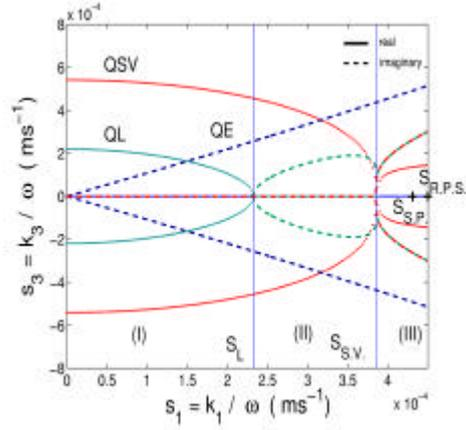
Fig. 7. Generalized slowness curves for (001)-[100] PZT4 layer.
