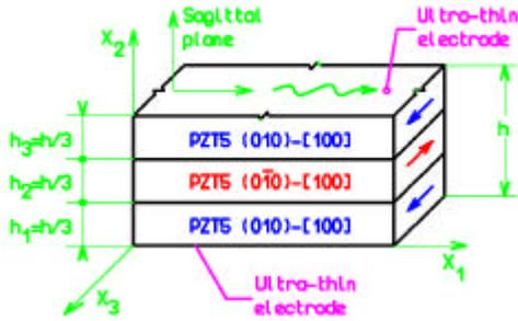
Fig. 1. Infinite piezoelectric sandwich plate in PZT5: geometry and notations.
