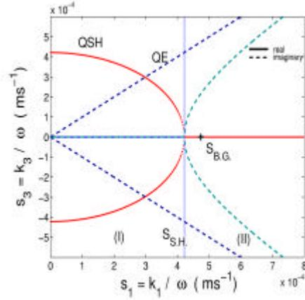
Fig. 4. Generalised slowness curves for (010)-[100] PZT5 layer.
