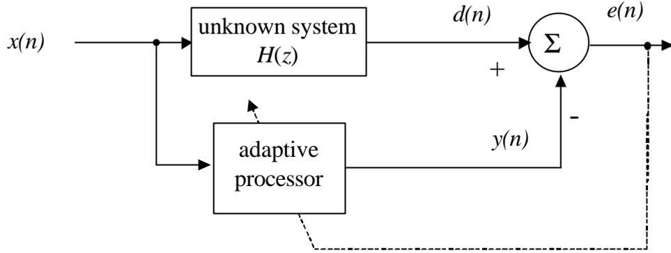
Fig. 1. Adaptive system modeling
