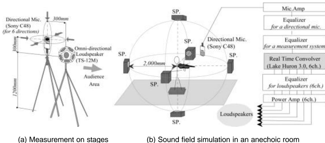
Fig. 1.- Outline of the 6-channel sound field simulation system
