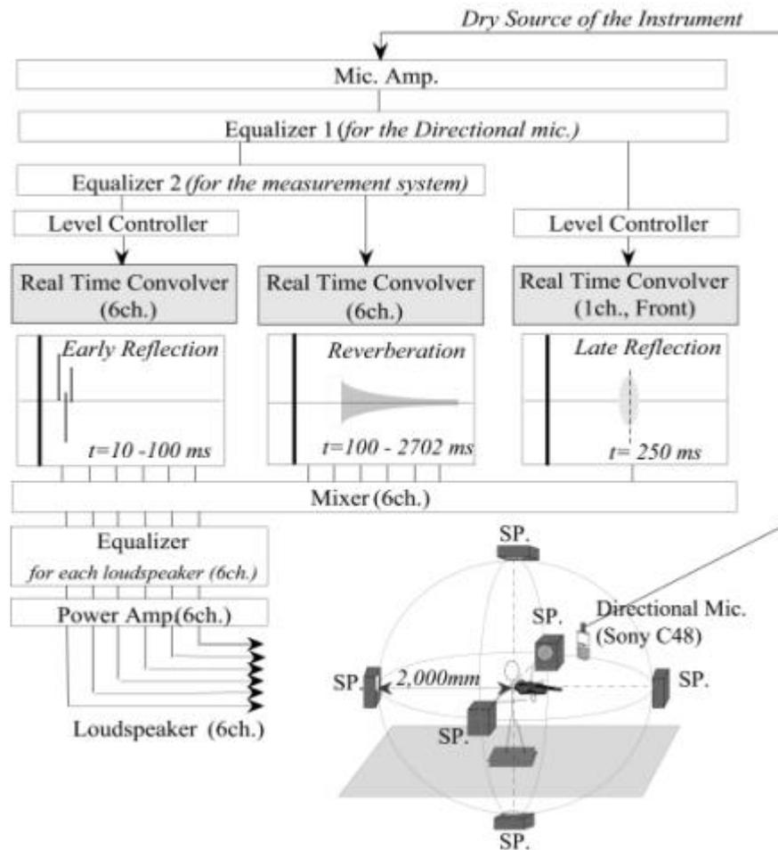
Fig. 2.- Block diagram of the simulation system for subjective experiment
