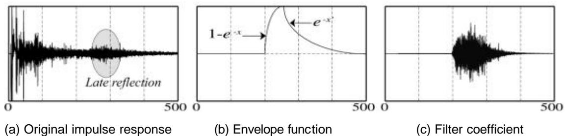
Fig. 3.- Processing the filter coefficient of late reflection
