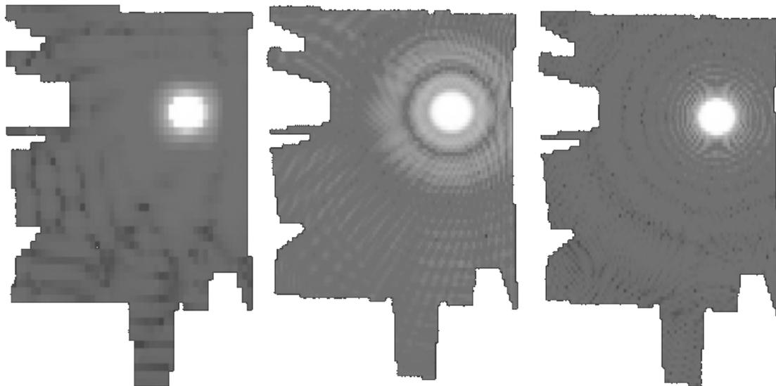
Fig. 6. SPL distribution for frequencies: 250, 1000 and 4000 Hz (left to right).
